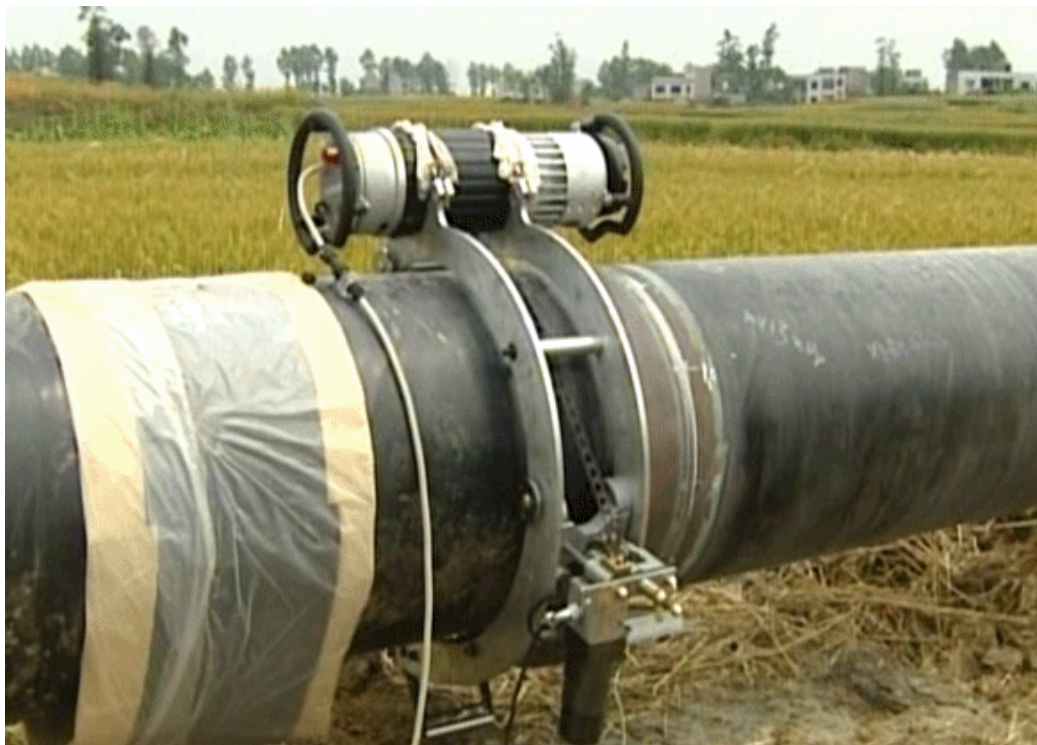
Drawing 3 Natural Gas Steel Pipe X-Ray Digital Imaging Detection
