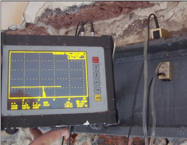
Figure 1. Readings on 3 mm reference hole
