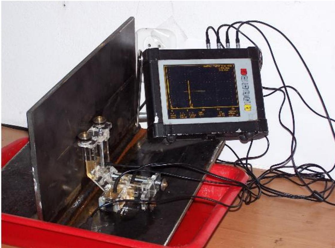
Figure 5. Angle weld tested by "Riksz", acceptable reading is shown on flaw detector's
