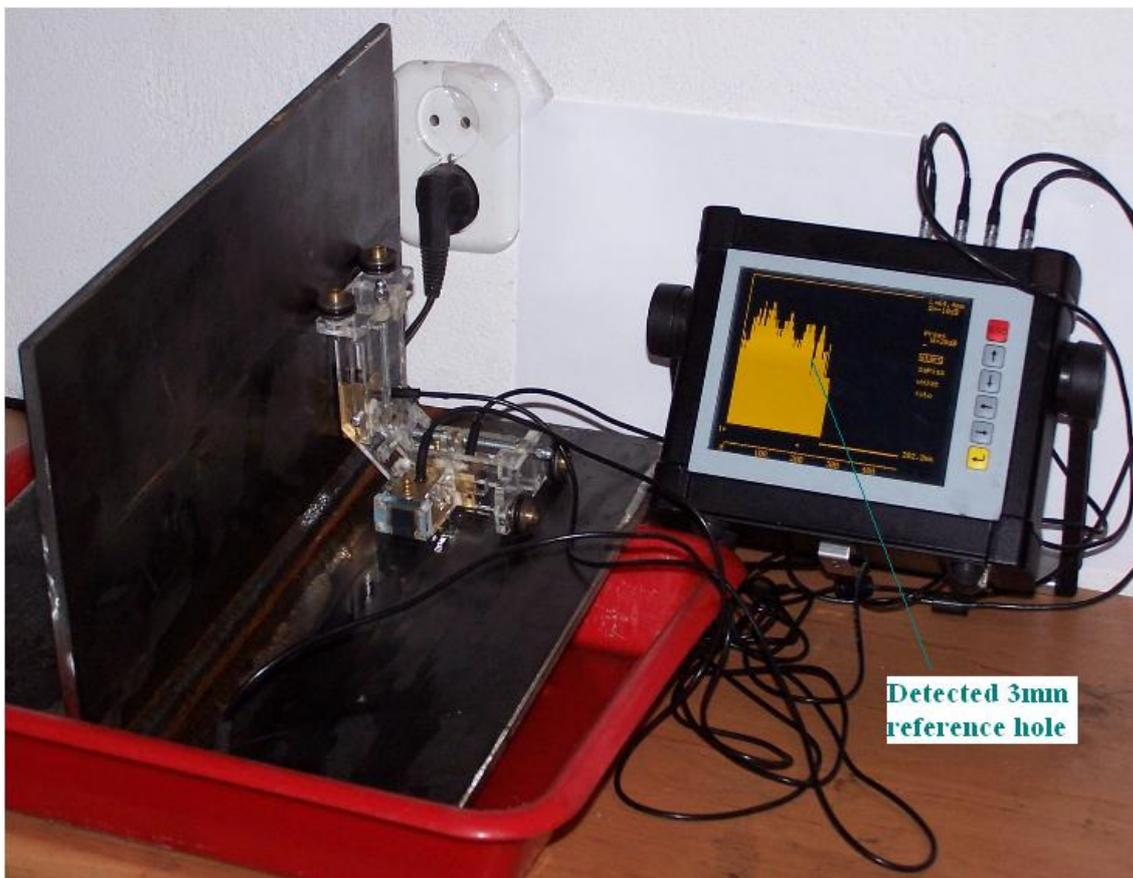
Figure 6. Angle weld tested by "Riksz", whole weld testing result is shown on flaw
