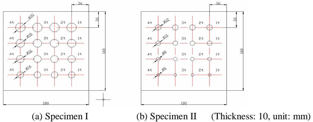
Fig. 3 Artificial specimens with back-drilled-bottom plate defects
