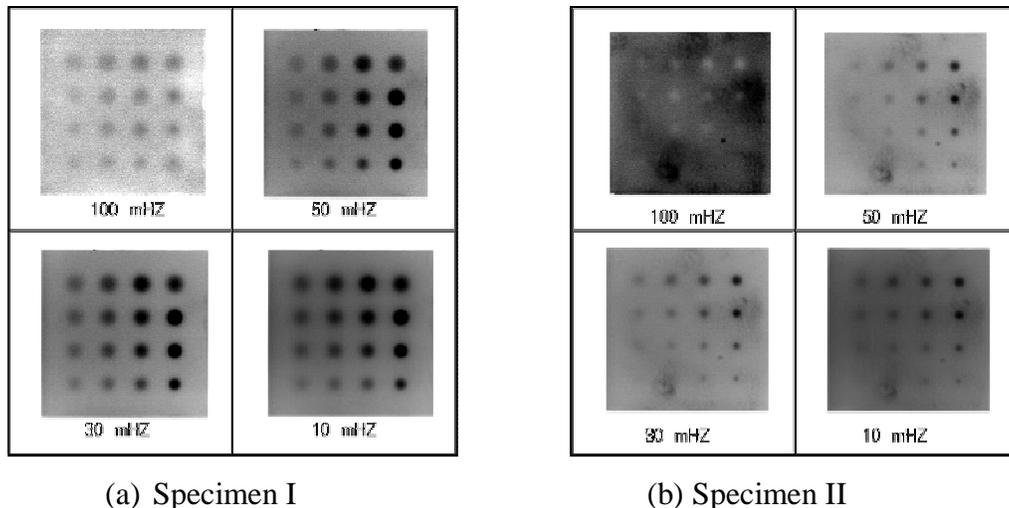
Fig. 6 Defect detection of SUS304 to each frequency
