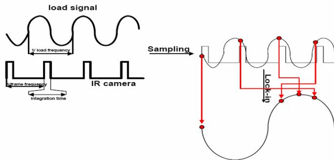
Fig.1 Signal processing of lock-in infrared thermography and system
