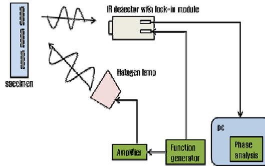
Fig. 4 Lock-in thermography system
