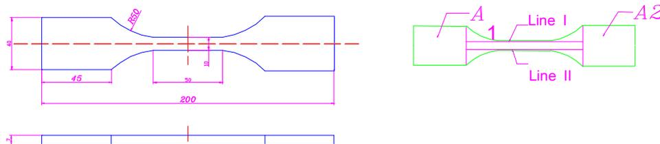
Fig1 The form of fatigue specimen and magnetic memory testing
