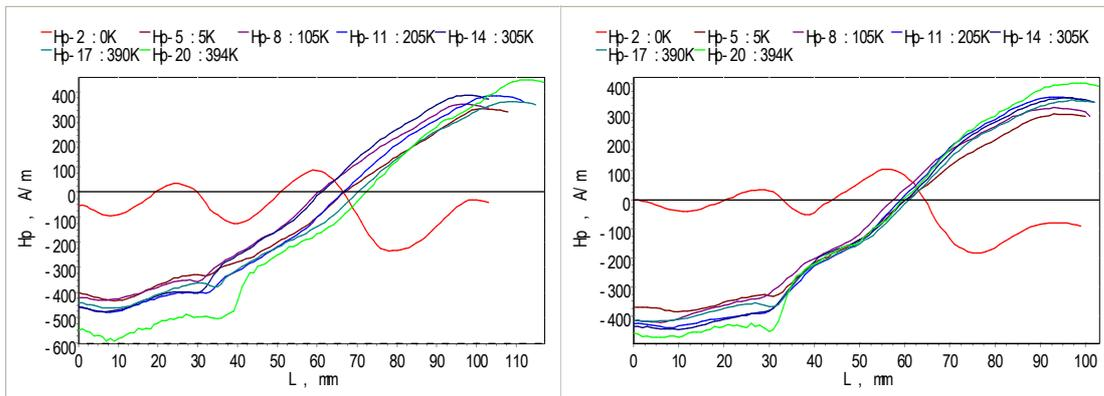
Fig5 MMT curve in the plane vertical magnetic vector about specimen with welded joint
