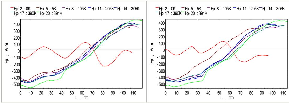
Fig2 MMT curves in horizon plane about specimen with welded joint
