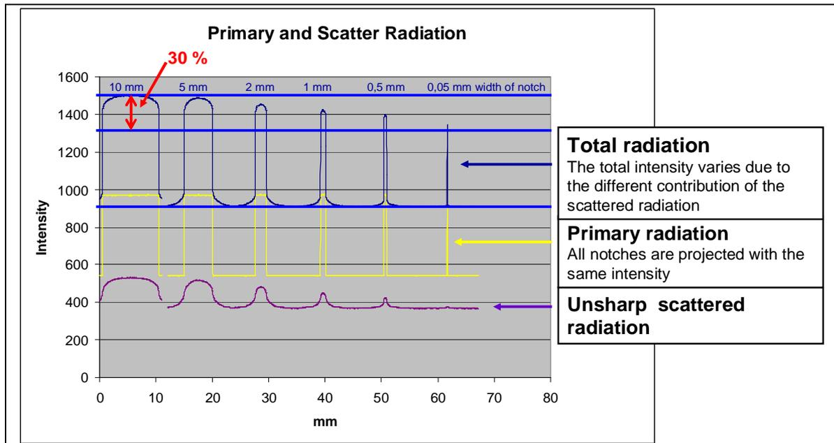
Fig. 3: Profiles of calculated contributions from scattered and primary radiation. The scattered radiation enhances the total contrast by about 30% for the wide notches and is negligible for the finest notches. Calculation for a 10 mm thick steel plate and 2 mm notch depth.
