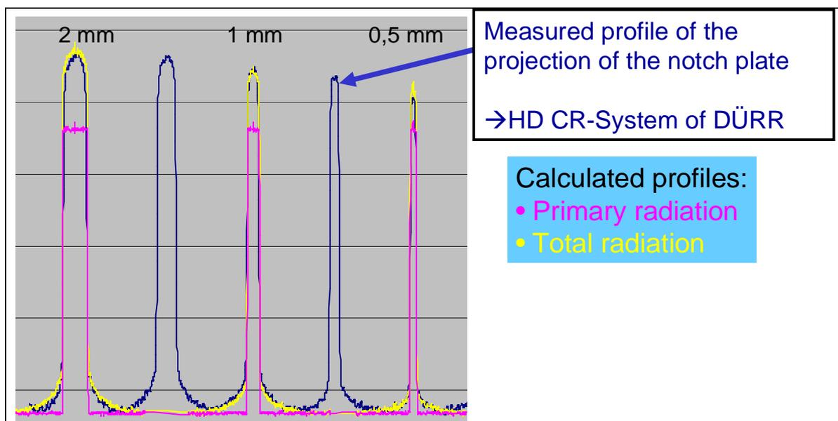
Fig. 4: Comparison of calculated and measured profiles of the notch plate for 2 mm, 1 mm and 0.5 mm wide and 2 mm deep notches.
