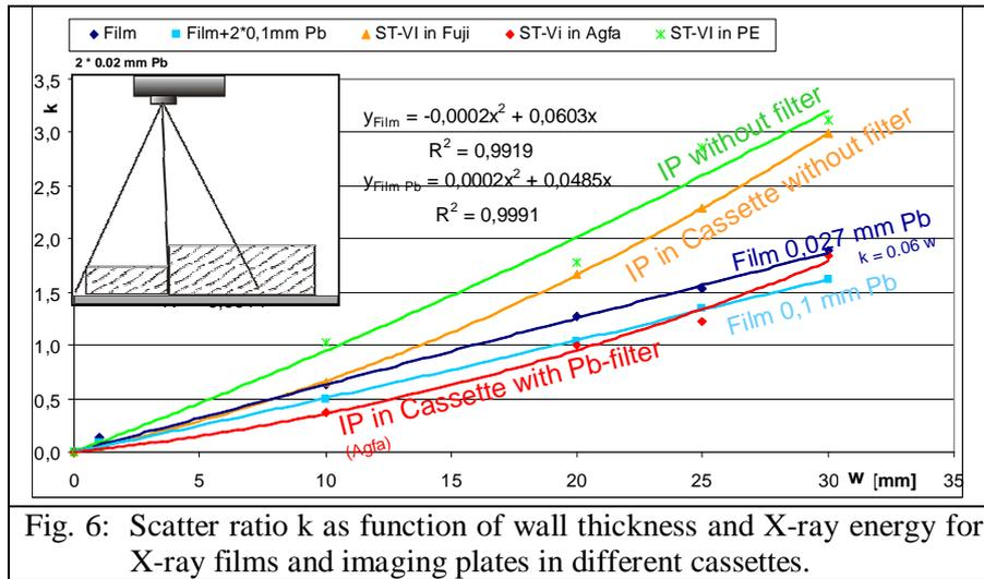
Fig. 6: Scatter ratio  $k$  as function of wall thickness and X-ray energy for X-ray films and imaging plates in different cassettes.
