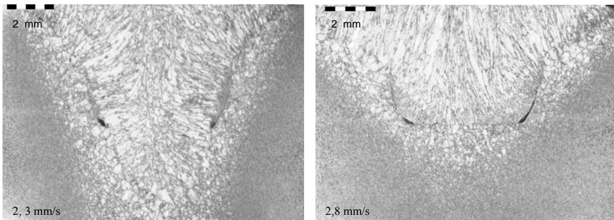
Fig. 7. Comparison of macro sections obtained with different welding speeds
