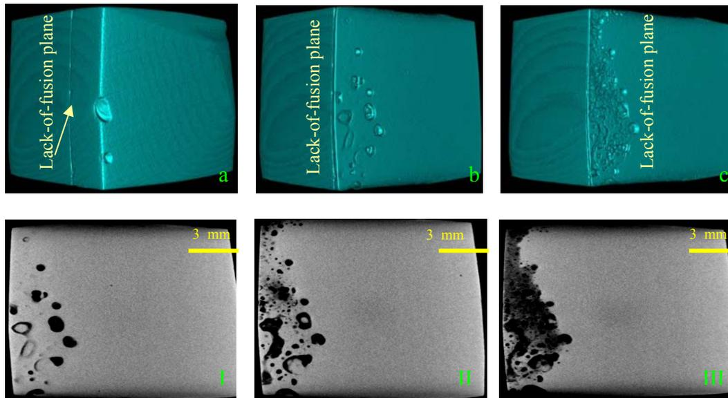
Fig. 6. Space (a,b,c) and planar CT images (I, II, III) of lack of fusion.
