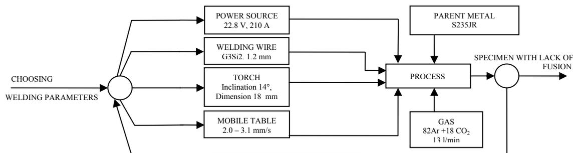
Fig. 2. Scheme of welding process
