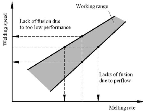
Fig. 1. Range of limited welding speed [4]
