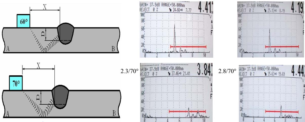
Fig. 3. Ultrasonic testing of weld and determination of lack-of-fusion location and size
