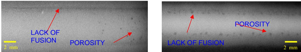
Fig. 4. X-ray images of welds 2.3 (left) and 2.8 (right)
