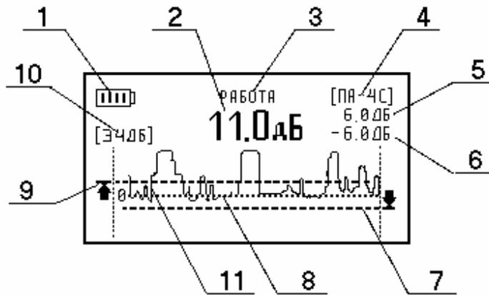
1 – battery; 2 – signal; 3 – operation mode; 4 – transducer type; 5 – upper threshold; 6 – lower threshold; 7 – lower threshold line; 8 – reference level line; 9 – upper threshold line; 10 – scale; 11 – signal oscillogram.
