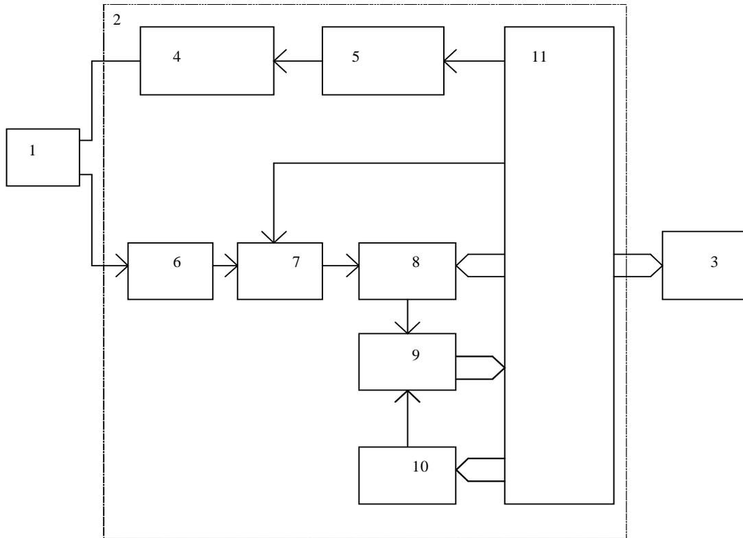
1 – transducer; 2 – electronic unit; 3 – PC (laptop); 4 – exciter; 5 – driving generator; 6 – front amplifier; 7 – variable bandwidth filter; 8 – programmable filter; 9 – ADC; 10 – programmable timer; 11 – interface.
