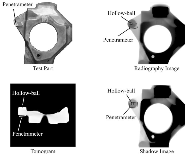
**Figure 7: The radiography image and its corresponding shadow image and one tomogram of the test part.**
