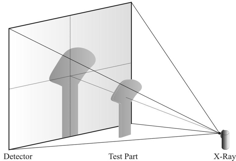
**Figure 1: Typical perspective geometry of a radiography system.**
