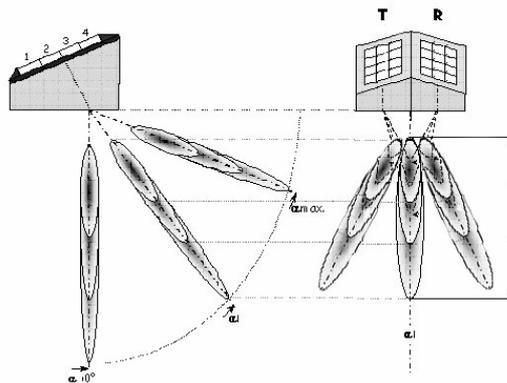
Figure 3: Schematic showing typical TRL-PA probes.
