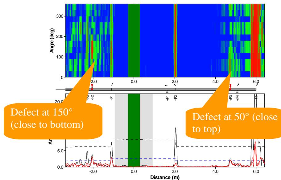
Figure 8. Typical screen for unrolled pipe C Scan
