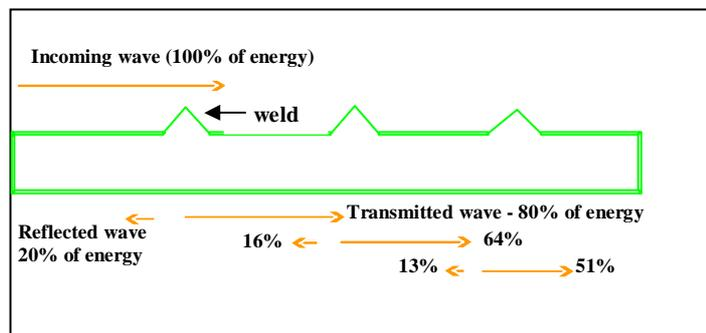
**Figure 2.** Schematic of wave behavior in the presence of welds
