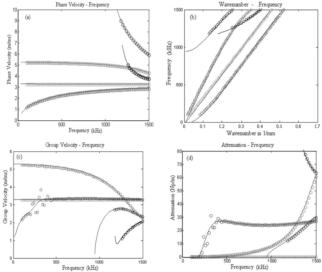
**FIGURE 2.** Dispersion curves of phase velocity (a), wavenumber (b), group velocity (c) and attenuation (d) of 1mm steel cylinder bar immersed in water predicted by SAFE method (o) and DISPERSE (—).
