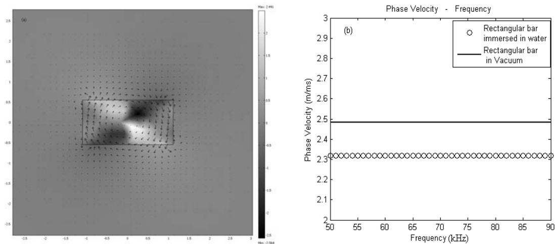
**FIGURE 3.** Theoretical prediction of mode shape of torsional mode of aluminium bar with rectangular cross-section (1.1mm\*2.2mm) immersed in alcohol at 50KHz (a) and dispersion curves of phase velocity (b)
