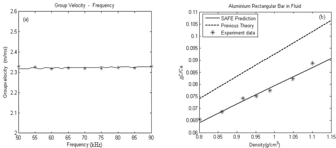
**FIGURE 5.** Measured (\*) and theoretically predicted (—) group velocity of aluminium bar with rectangular cross-section immersed in alcohol (a) and different fluids (b)
