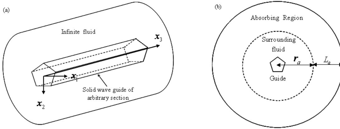
**FIGURE 1.** Schematics of (a) 3D solid waveguide immersed in a fluid and (b) 2D model with absorbing region used for FE simulation of system shown in (a)
