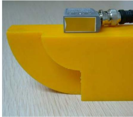
Fig. 9 Probe with angled wedge and test block made from PE
