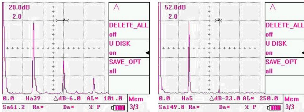
Fig.5 Attenuation of steel and polythene
