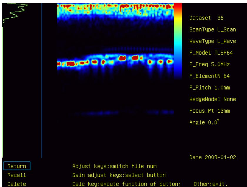
Fig. 12 Ultrasound phased array inspection for heating wire dislocation
