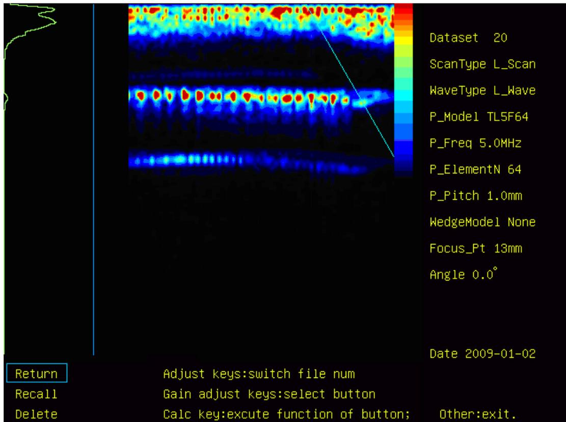
Fig. 14 Electro-fusion joints phase transition line
