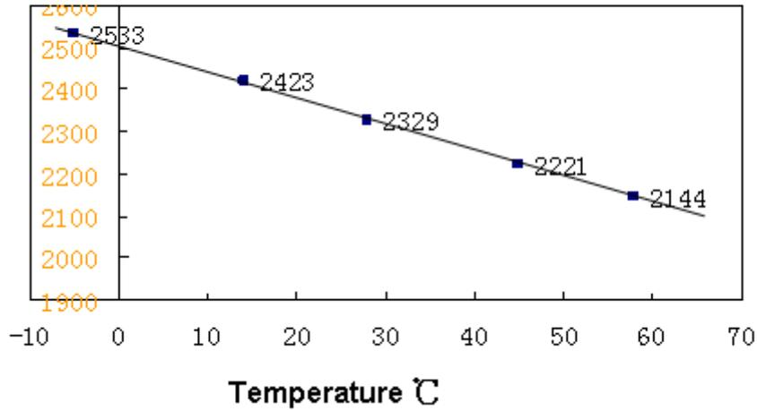
Fig.6 Velocity change with temperature
