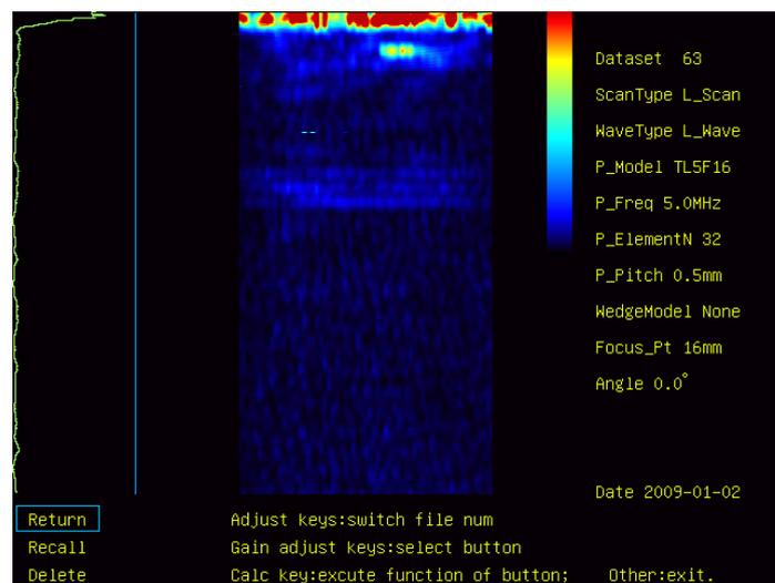
Fig. 15 Ultrasound phased array inspection for good heat fusion joint
