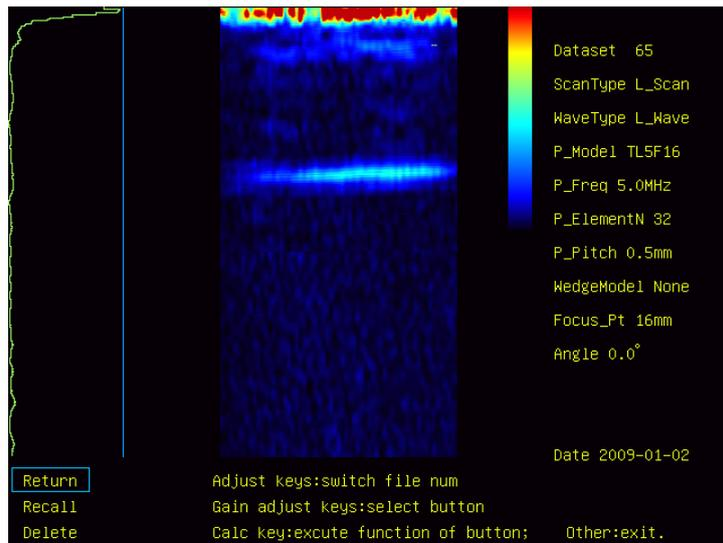
Fig. 16 Ultrasound phased array inspection for bad fusion on heat fusion joint face
