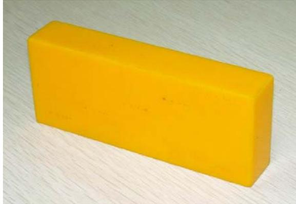
Fig. 17 Test block for PE pipe ultrasound phased array inspection
