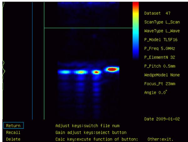
Fig. 13 Ultrasound phased array inspection for gas holes
