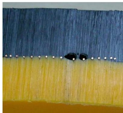
Fig. 2 Fusion line with gas holes
