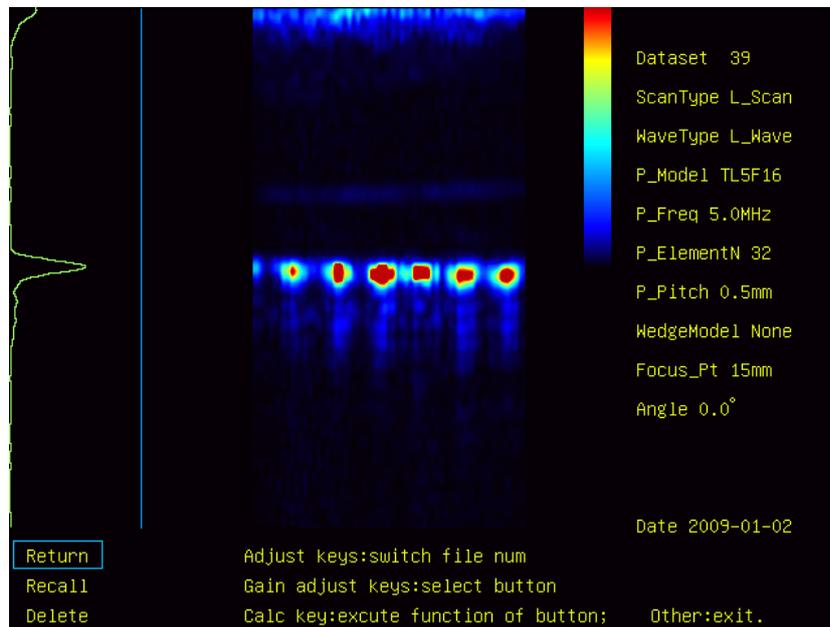
Fig. 11 Ultrasound phased array inspection for good fusion joint
