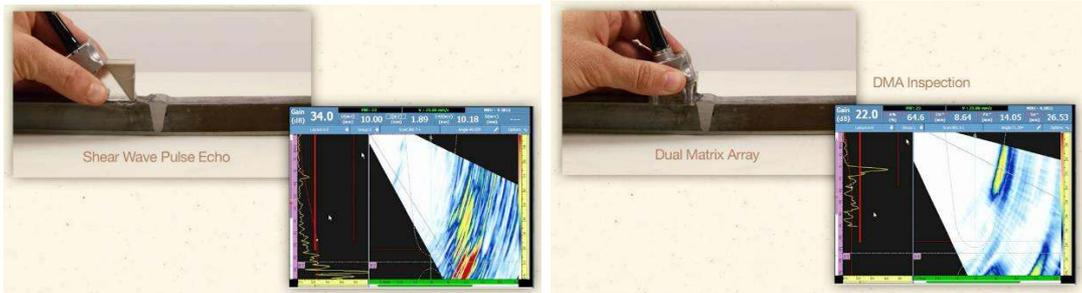
Figure 4: Illustration of the efficiency of the DMA solution for CRA-Clad weld inspection. Left: SW phased-array probe; Right: DMA probe
