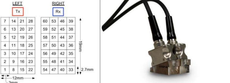
Figure 3: Left: DMA(Dual Matrix Array) probe configuration; Right: DMA probe picture
