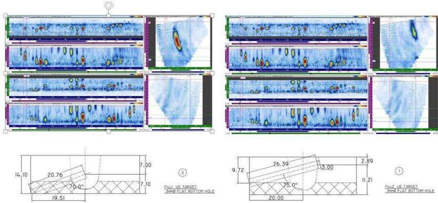
Figure 11: PipeWizard imaging of the pipeline segment illustrating volumetric flaws detection
