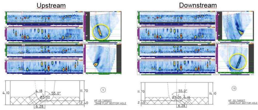
Figure 12: PipeWizard imaging of the pipeline segment illustrating hot passes flaws detection
