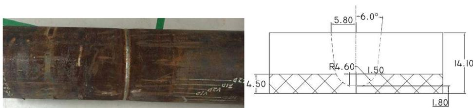
Figure 8: Picture of pipeline segment and J-Weld cross section schematic
