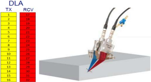
Figure 2: Left: DLA(Dual Linear Array) probe configuration; Right: DLA probe operation mode
