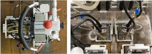
Figure 9: Olympus equipment for DLA inspection. Left: PipeWizard scanner; Right: DLA probes mounted on the scanner
