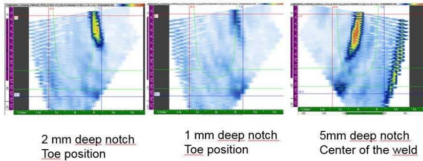
Figure 13: Detection of different surface notches
