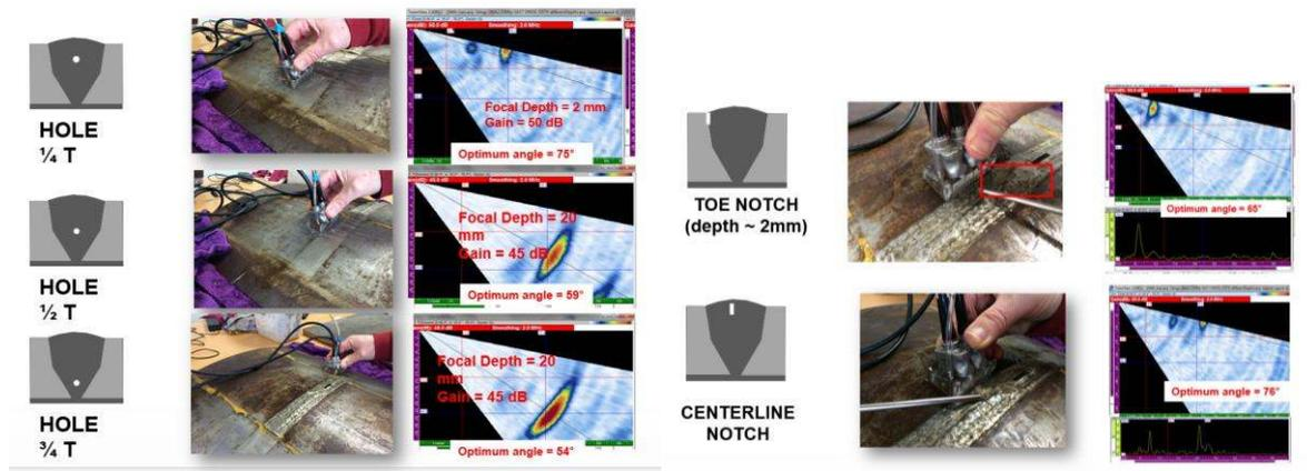
Figure 7: Results obtained for volumetric reflectors (left) and surface notches (right)
