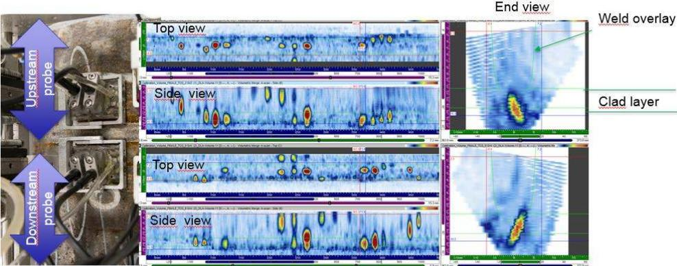
Figure 10: PipeWizard imaging of the pipeline segment illustrating root flaws detection
