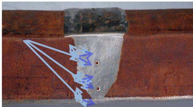
Figure 1: Effect of the anisotropic structures of the weld and cladding on shear wave ultrasonic beams
