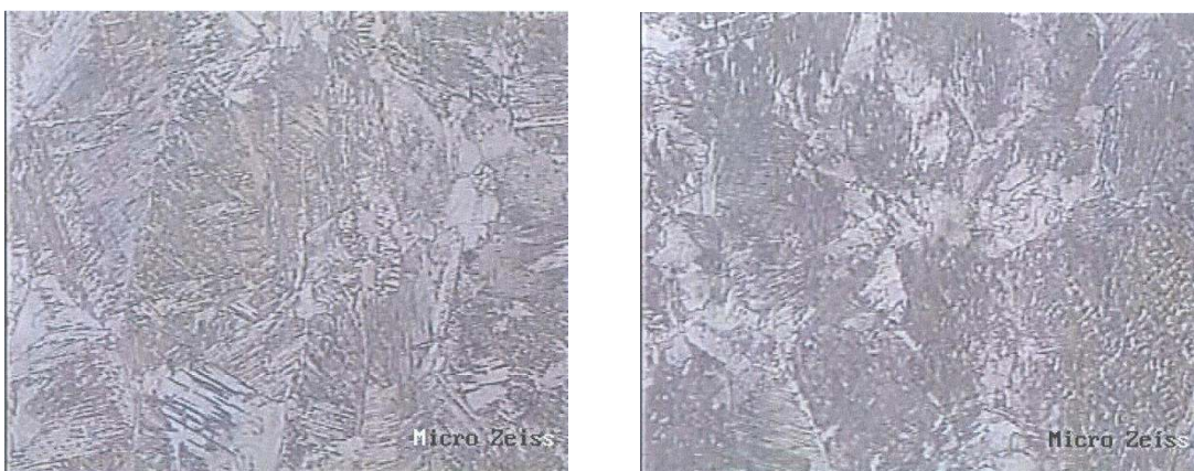
Fig 5: Micrograph showing micro structure in low carbon steel thickness 0.8 mm (45 and 47 KA)
