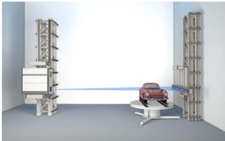
**Fig. 2.** Mechanical setup of the XXL-CT system.
