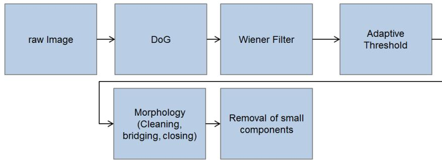
**Fig. 2.** Defect extraction from CT data – image processing algorithm.
