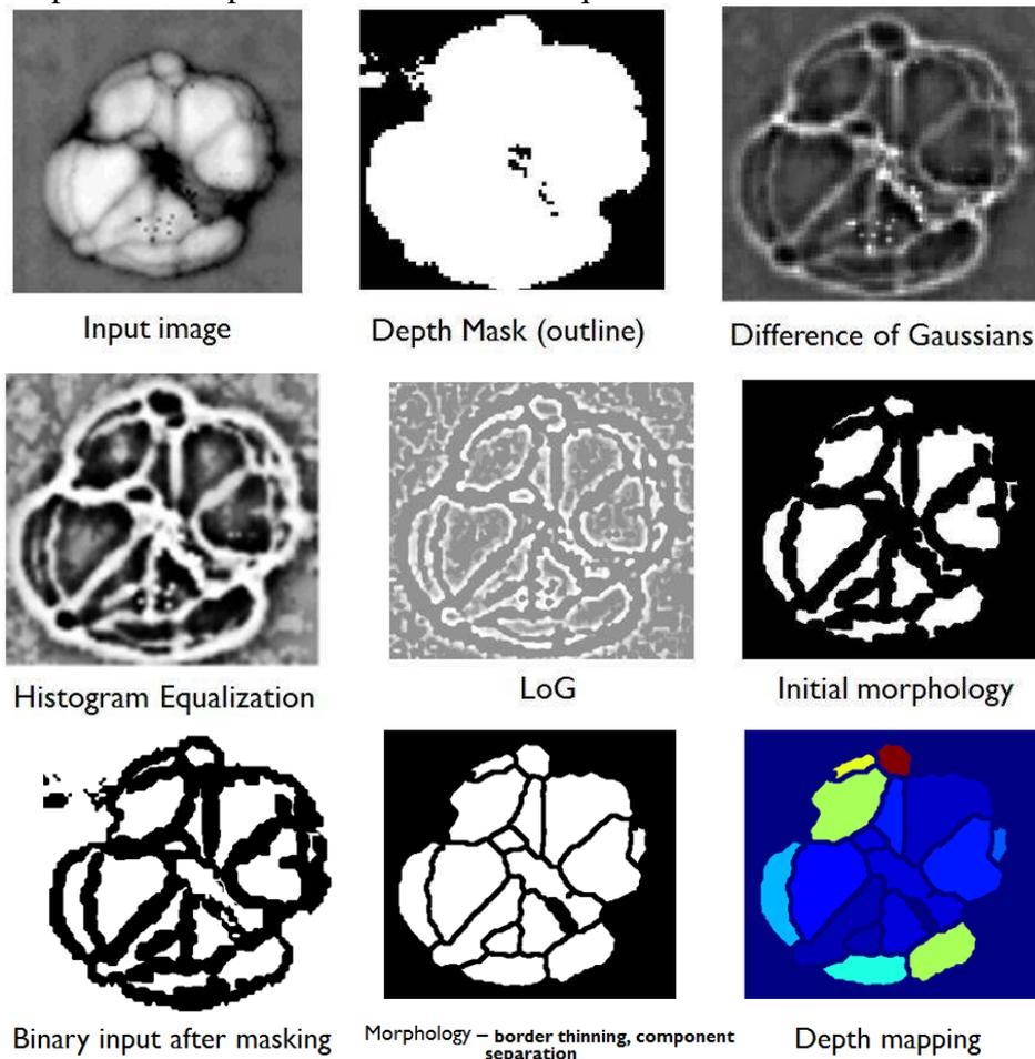
Fig. 8. Image processing of ultrasonic C-Scan data – interim steps.
