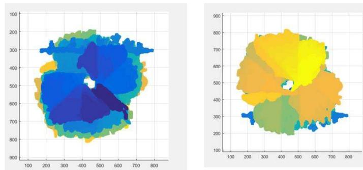
**Fig. 5.** Resultant delamination – top projection, analog to ultrasonic C-Scan.
