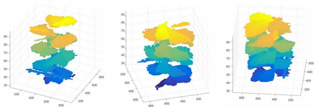
**Fig. 4.** Resultant delamination – voxel set obtained from CT data processing.
