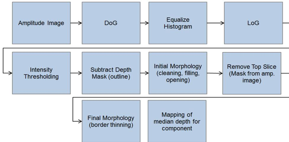
Fig. 7. Image processing of ultrasonic C-Scan data.
