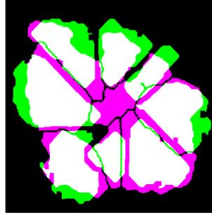
**Fig. 10.** CT and ultrasonic C-scan – extracted patches overlay
