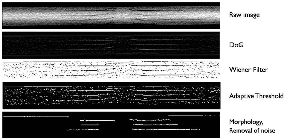
**Fig. 3.** Defect extraction from CT data – interim steps.
