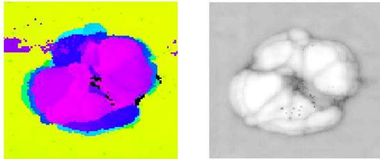
**Fig. 1.** Ultrasonic C-scan of a delamination used in the present study – time of flight (depth), amplitude .
