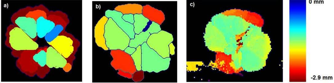
**Fig. 9.** Qualitative comparison a) features extracted from CT, b) features extracted from UT, c) raw UT data (time-of-flight).
