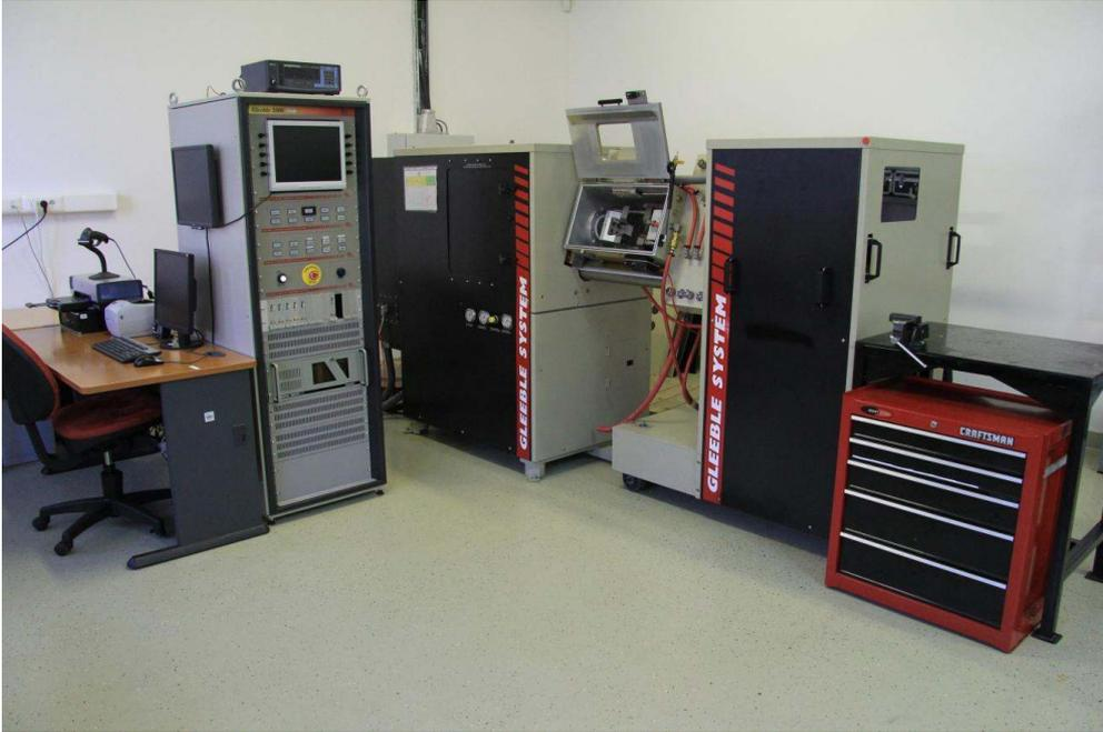
Fig. 1. Gleeble 3800 thermo-mechanical simulator with an open experimental box.
