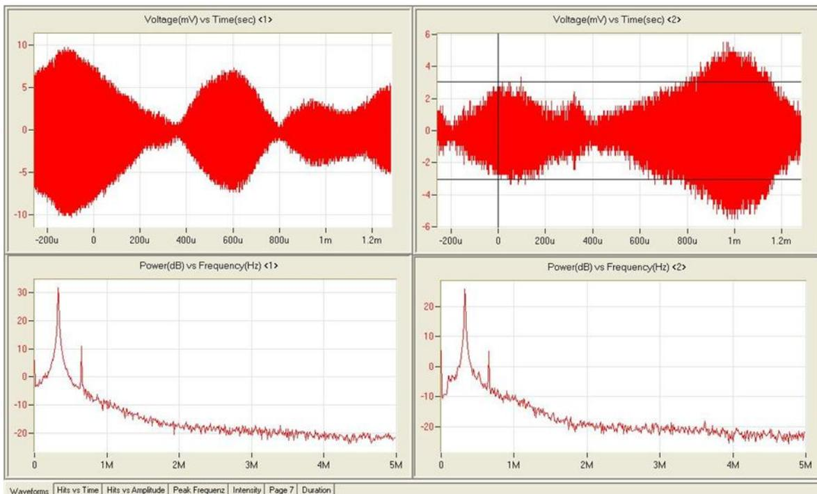
**Fig. 8.** Acoustic emission analysis during the induction heating
