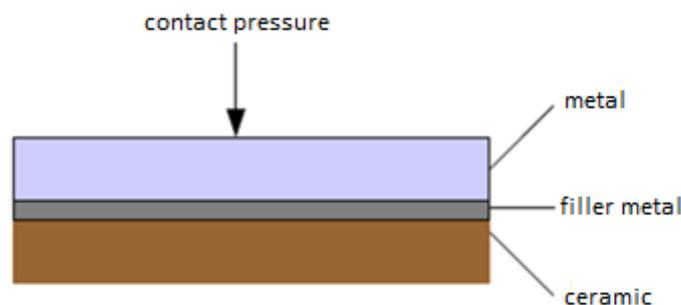
**Fig. 1.** Principle of the reactive air brazing (RAB).
