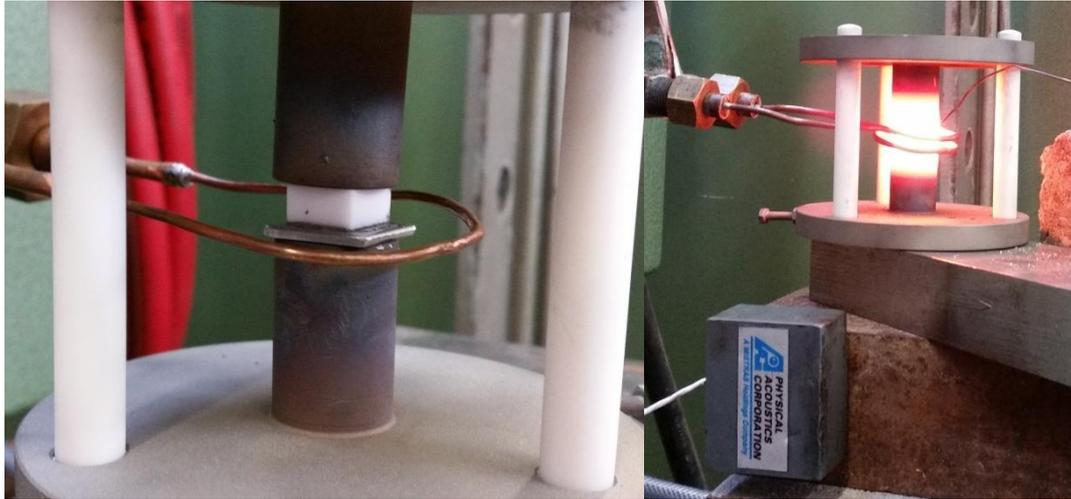
**Fig. 7.** Experimental setup (left: before brazing, right: during brazing).
