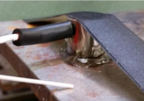
**Fig. 4.** Calibration by cracking a ceramic sample
