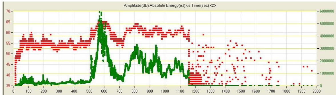
**Fig. 9.** Acoustic emission analysis during the brazing process
