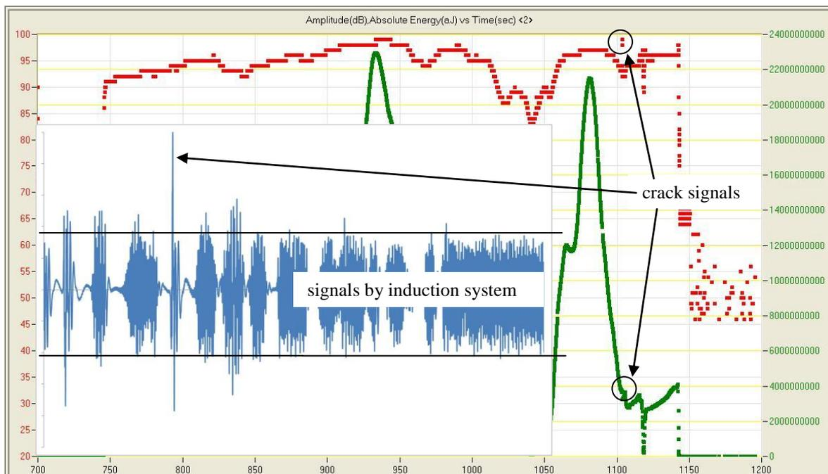
**Fig. 10.** Acoustic emission analysis during the brazing process
