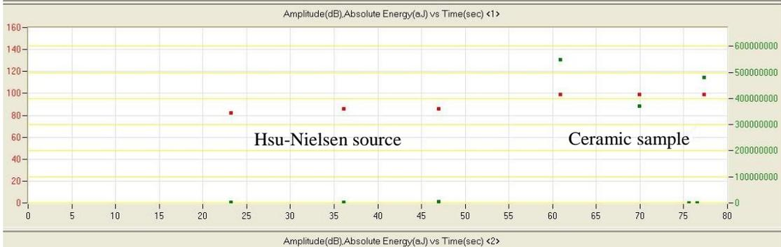
**Fig. 5.** Comparison of the Hsu-Nielsen source and the ceramic sample.
