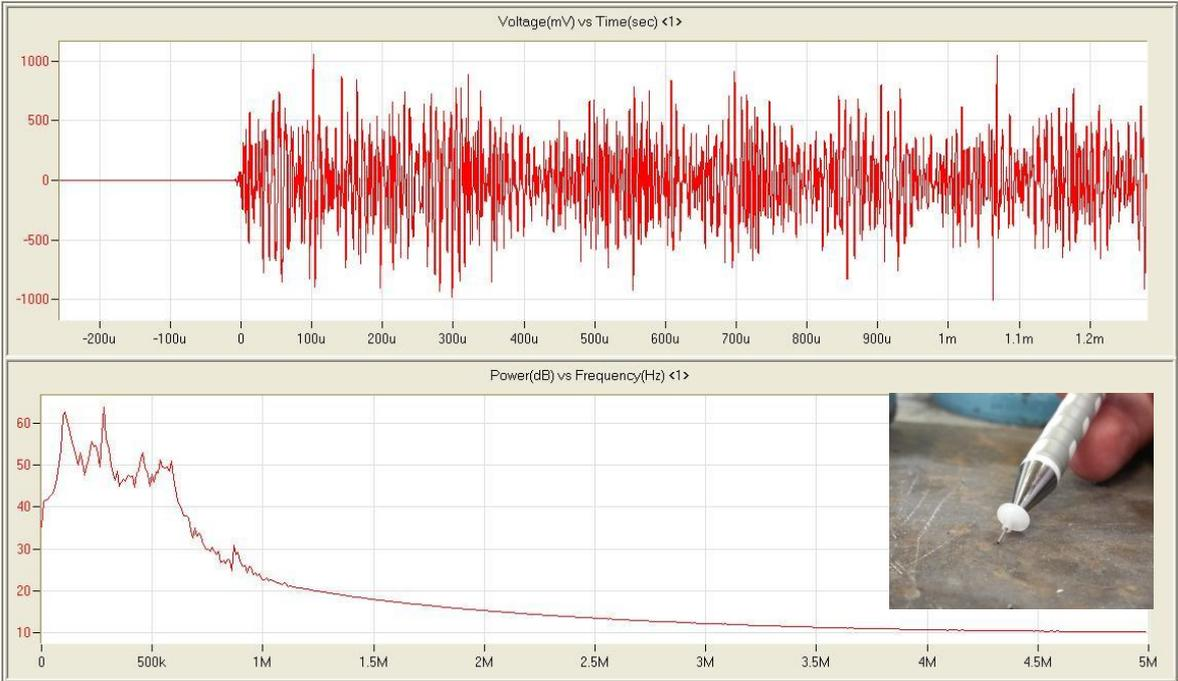
Fig. 3. Result of the function test by using a Hsu-Nielsen source.
