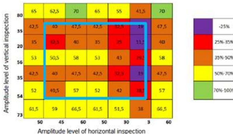
**Fig 6.** Severity estimation of wall loss under a compensation pad based on signal amplitude levels
