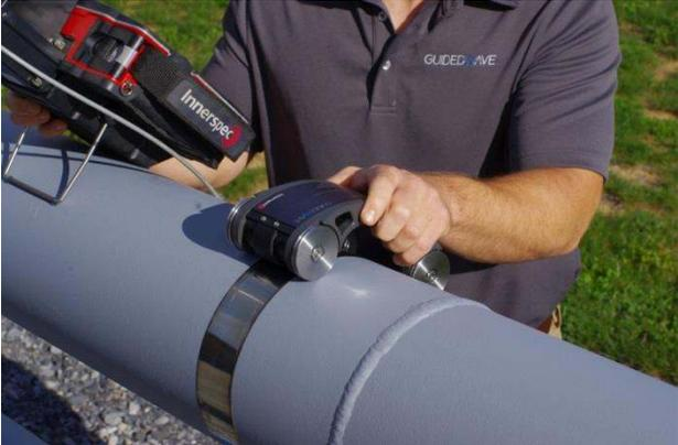
**Fig 8.** Circumferential scanning with magnetostriuctive sensor
