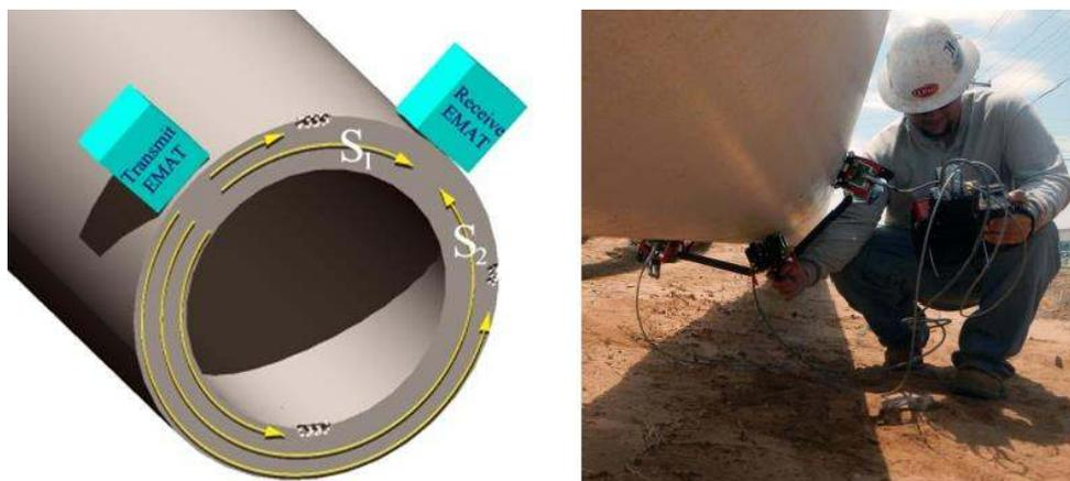
**Fig 3.** Configuration for axial inspection in a pipe with MRUT guided waves
