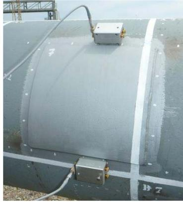
**Fig 4.** Transmitter and receiver probes located at both sides of a compensation pad
