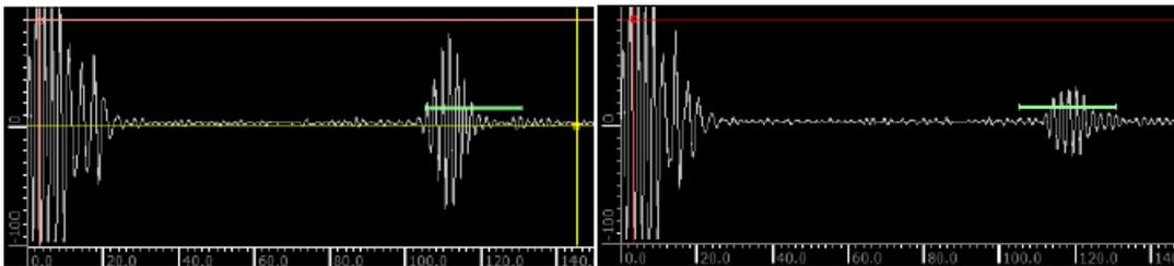
**Fig 5.** Oscilloscope image of a flawless area (left) and a defective zone (right)
