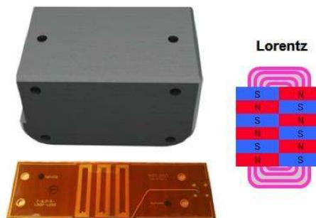
**Fig 2.** Configuration of coil and magnet used for generating shear horizontal guided waves
