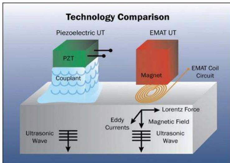
Fig 1. Technology comparison between piezoelectric UT and EMAT
