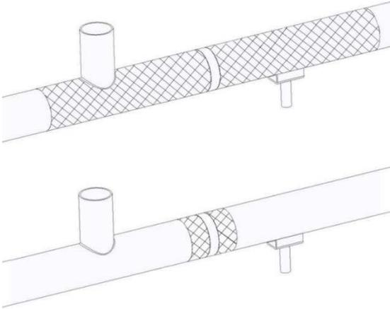
**Fig 9.** LRUT (up) and MRUT (down) dead zones comparison
