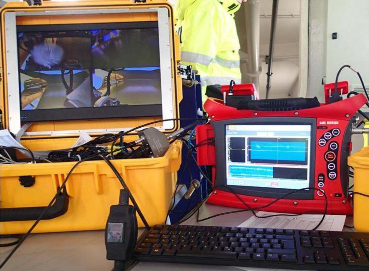
Figure 9: Control area with PA-Unit (Gekko) and Video Monitor
