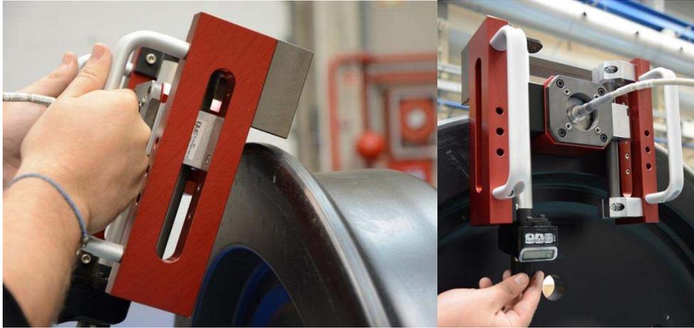
Figure 7 Stress sensor mechanical sensor positioner
