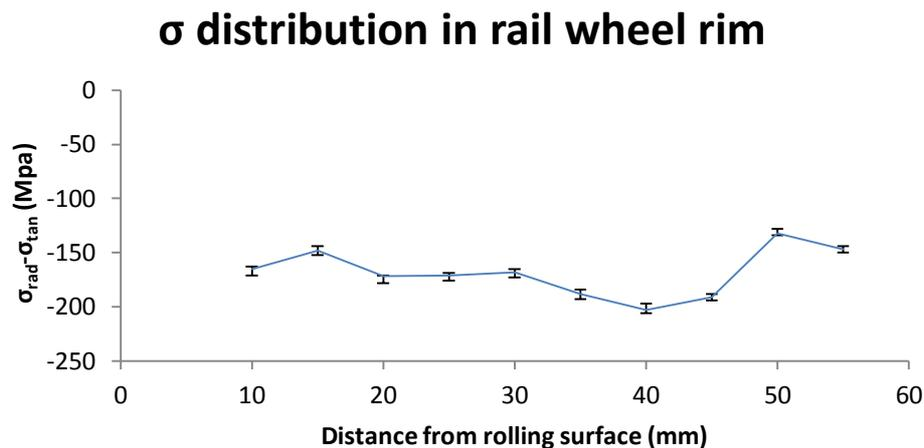
Figure 8 Residual stress distribution and measurement error in sample rail wheel
