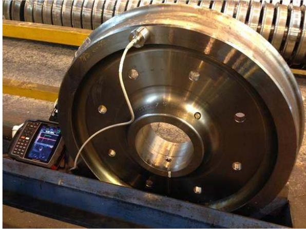
**Figure 3** Innerspec PowerBoxH performing stress measurement on rail wheel
