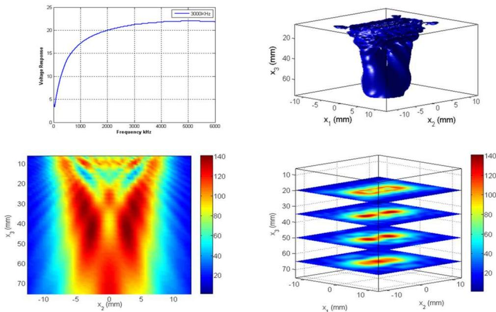
**Figure 4** Frequency Spectra & 3dB Beam Profiles for one coil (sensor contains two orthogonal coils)
