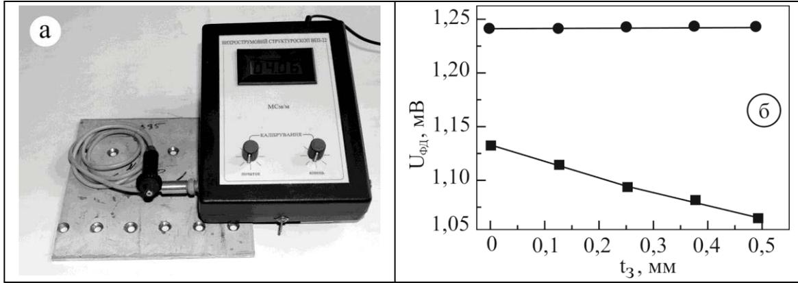
**Fig. 6.** Eddy current conductivity meter VEPR-22 (a) and the dependence of the output voltage on the lift-off distance  $t_z$  without lift-off suppression (■) and with suppression algorithm application (●) (b).
