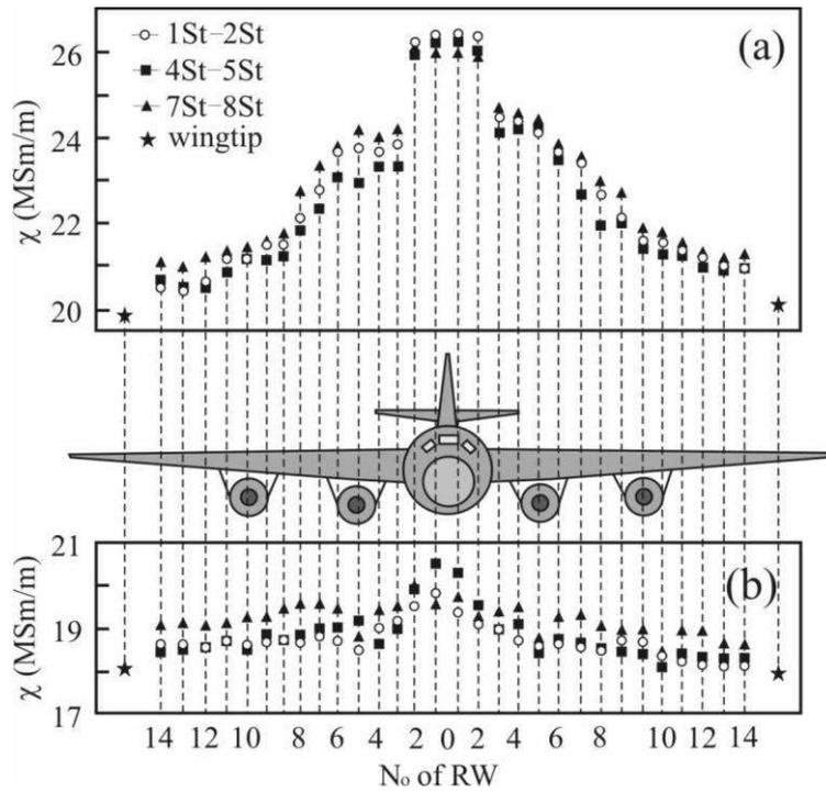
**Fig. 7.** The change of material conductivity in various areas of (a) upper (B95T1 alloy) and (b) bottom (D16ATHB alloy) wing and center section skins of AN-12 type aircraft after long-term exploitation.
