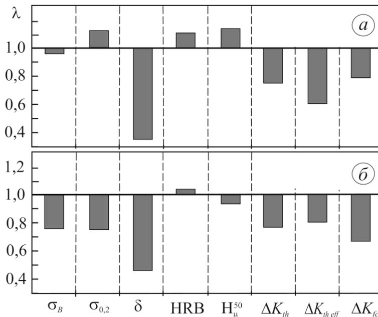
**Fig. 1.** The influence of simulated degradation on the mechanical characteristics of D16 (a) and B95 (b) aluminum alloys:  $\lambda$  - related characteristics of the material in its initial and degraded conditions.
