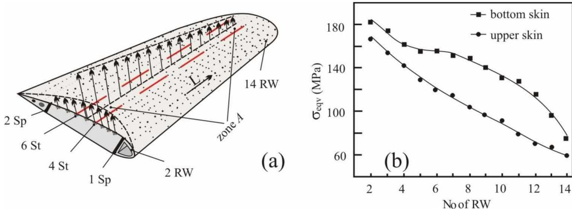
**Fig. 2.** Zone A of specimens cut out from aircraft wing skins (a) and (b) level of applied equivalent stresses in the bottom and upper skins: RW – rib of the wing; St – stringer; Sp – spar; L – sheet rolling direction.
