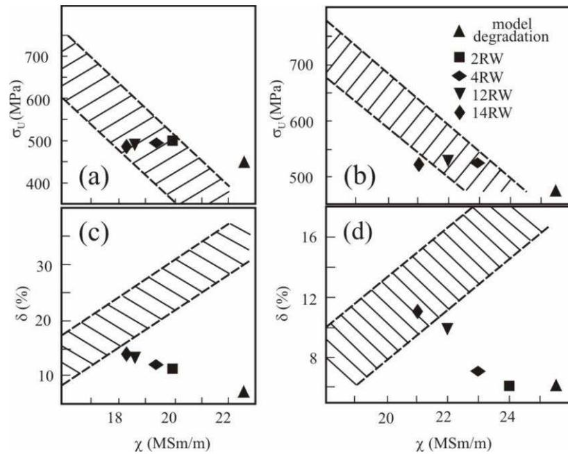
**Fig. 3.** Relationships between ultimate strength  $\sigma_U$ , elongation  $\delta$  and conductivity  $\chi$  of (a, c) D16 type and (b, d) B95 type aluminum alloys: dashed regions represent the literature data for alloys in as-received state; symbols are given for such alloys after long-term exploitation in areas from 2 RW to 14RW and after model degradation.
