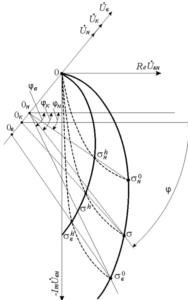
Fig. 5. Diagram of proposed EC algorithm for conductivity measurements with lift-off influence suppression.
