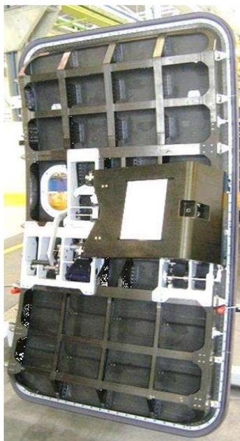
**Fig. 1.** Full composite prototype for a passenger door
