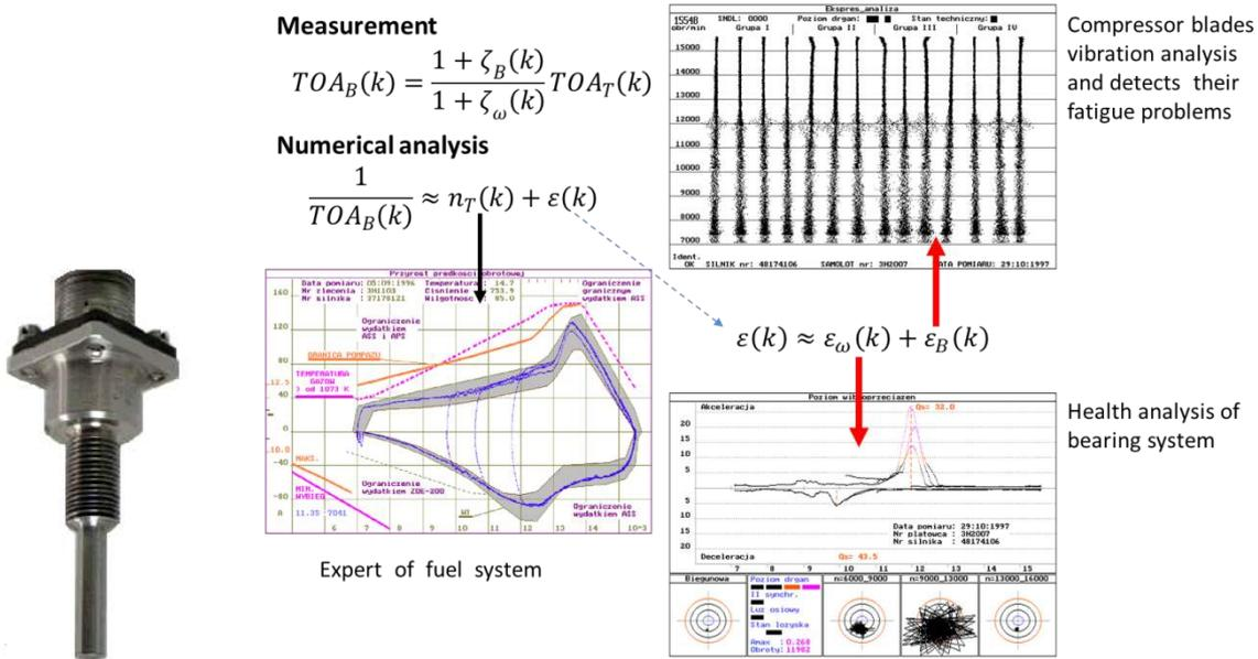
Fig. 4. Examples of VR sensor and imaging results on the phase plane (SO-3 engine,  $f_{clock} = 10$  MHz) [15]
