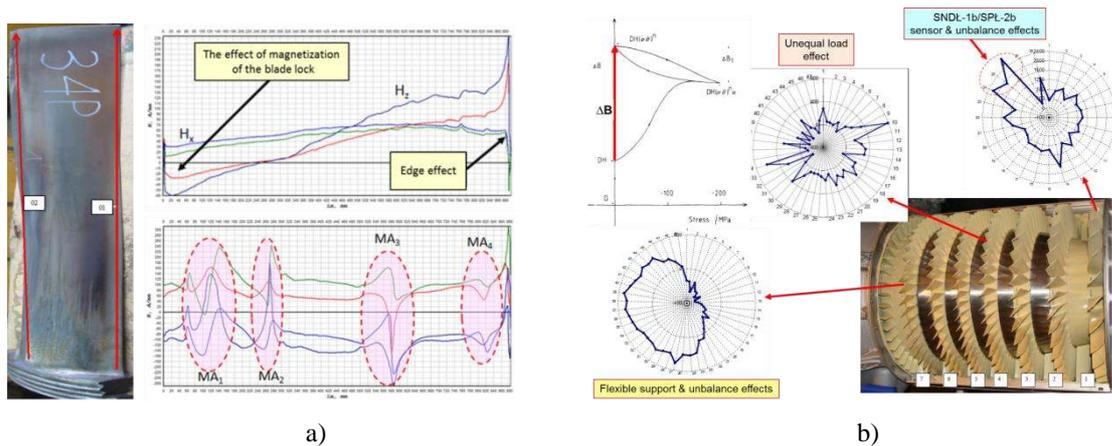
**Fig. 3.** The influence of an unknown load history on the magnetization of: a) LP blades of steam turbine (new blade and after overload,  $MA_i$  – the magnetic anomaly correlated with nodal line of vibration, the state before crack) [19]; b) compressor blades of jet engine SO-3 [3]
