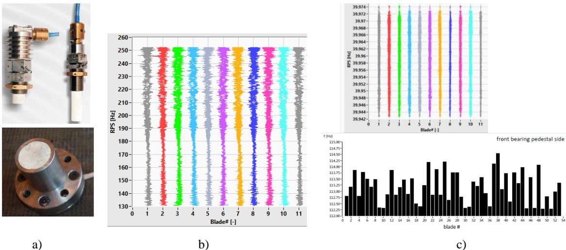
**Fig. 9.** Illustrated: a) high temperature metallic-ceramic VR sensors contain one and four coils (the top and bottom photo, respectively); b) vibration of turbine blades of turbofan engine RD-33 ( $f_{\text{clock}} = 200$  MHz); c) vibration of ND-37 blades of steam turbine 18K370 ( $f_{\text{clock}} = 100$  MHz)
