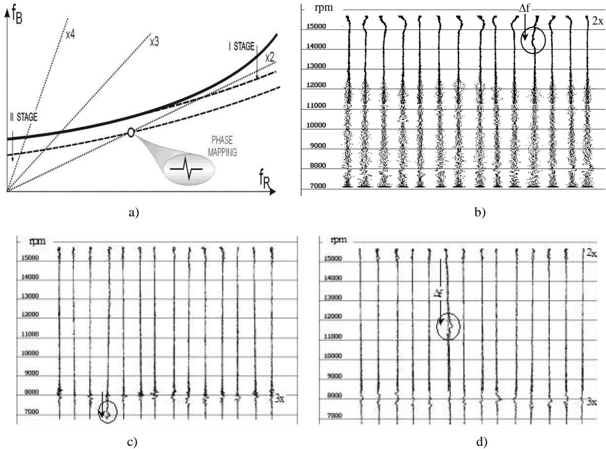
**Fig. 7.** The effect of blade cracking as phase representation of blade vibration [6]: a) blade frequency plotted in the Campbell diagram; b) cyclical weakness - first stage crack of blade fatigue, only decrease in  $B$  ratio growth dynamic frequency; c) second stage crack of blade – changes  $f_B(0)$  and  $B$ , signal after low band filtration; d) finish stage crack of blade – 5 minute before break, signal after low band filtration
