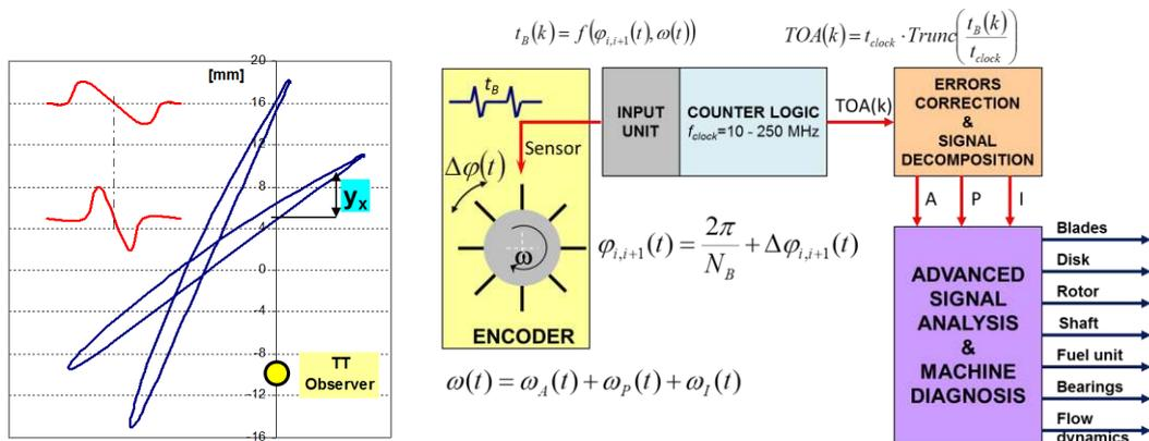
**Fig. 2.** Idea of the tip timing method (input unit includes low-band signal filter, preamp and Schmidt trigger; counter logic includes the standard frequency generator and counter; A – aperiodic component, P – periodic component, I – interference and noise,  $y_x$  – the impact of blade vibration to change the trigger point)
