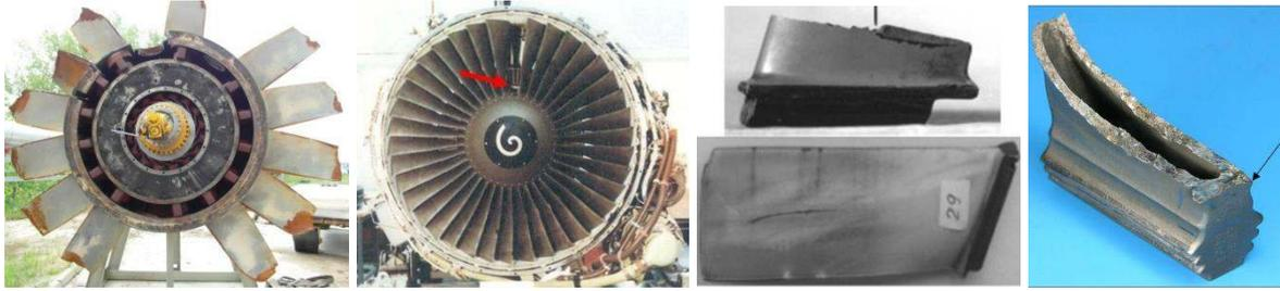
**Fig. 1.** Fatigue problems of fan, compressor and turbine blades [3, 4]
