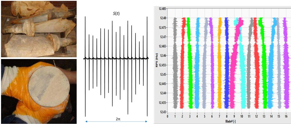
**Fig. 8.** Non-contact monitoring of fan blade flue gas desulphurisation plant ( $n_{\max} = 750$  rpm,  $f_{\text{clock}} = 80$  MHz)
