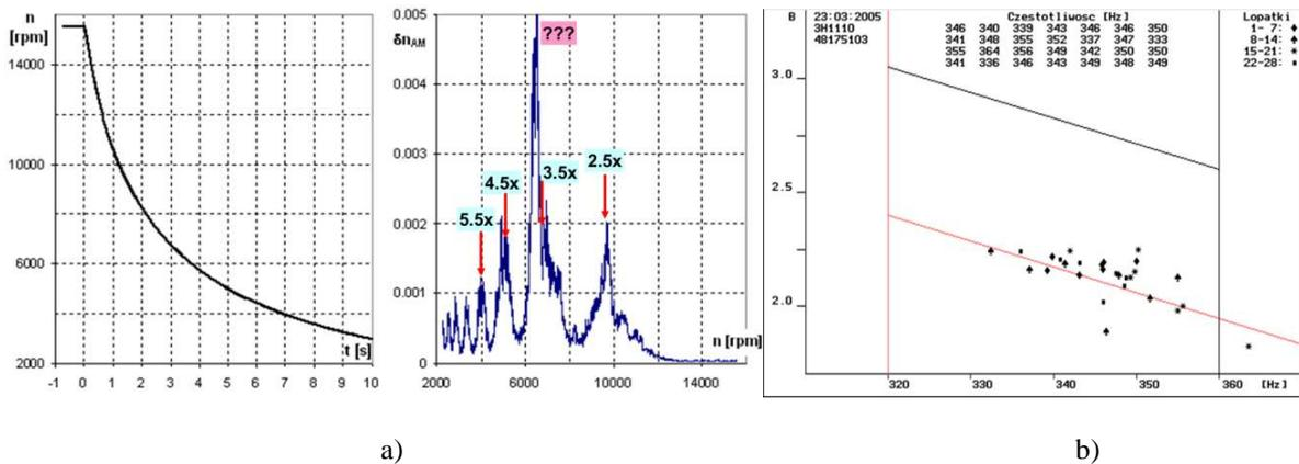
Fig. 5. Visualised [3,9]: a) identification of reaction order of blade vibration during dynamic transition states; b) aggregated result of the 1<sup>st</sup> mode's own vibration frequency  $f_{L,1}(0)$  and  $f_{L,1}(n) = f_{L,1}(0) + B \cdot f_n^2$
