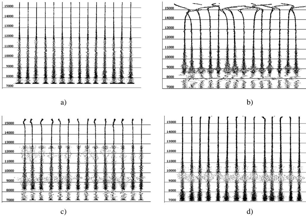
**Fig. 6.** Phase mapping of blade vibration and ratio of the SO-3 engine compressor [6]: a) normal stress level; b) synchronous resonance - influence of a foreign object in the compressor inlet; c) asynchronous resonance - influence of stall during acceleration; d) asynchronous resonance – influence of rotor resonant vibration
