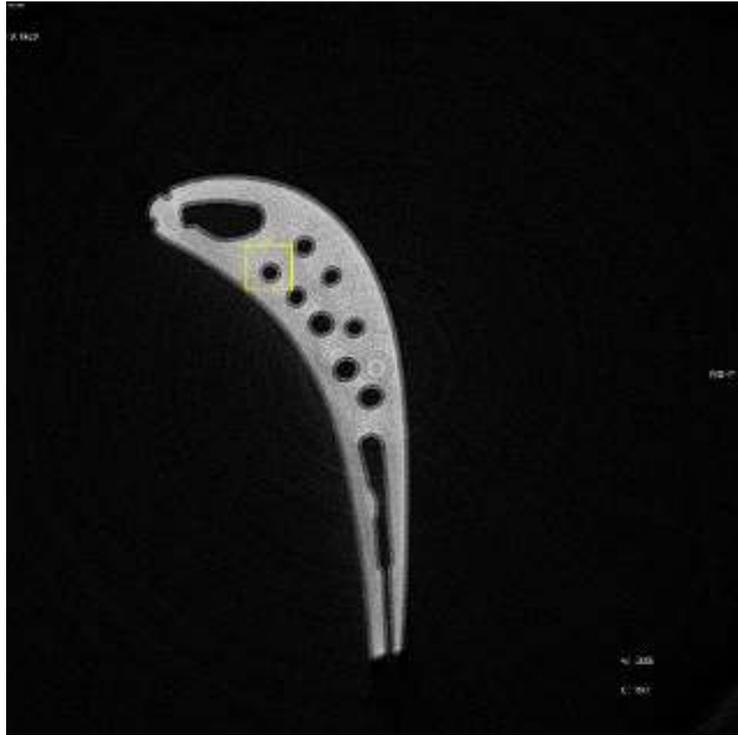
Figure 3 – Original image of Slice#0620 with ROI placed on Hole B
