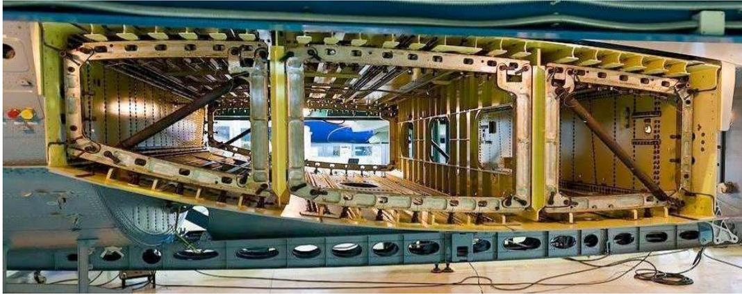
Fig. 1. Example of “unclosed” aircraft construction
