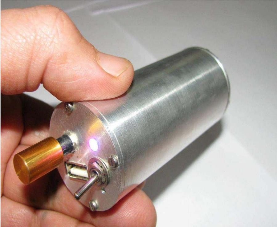
Fig.4 The ultrasonic leak tester "Koloran"
