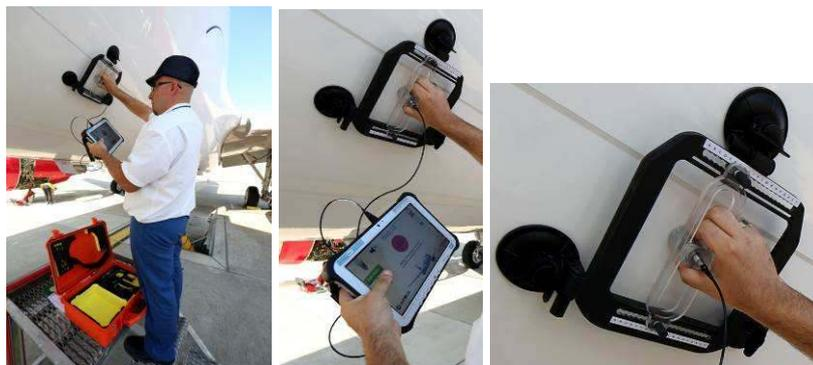
**Figure 16: Clad Tool hardware kit**
