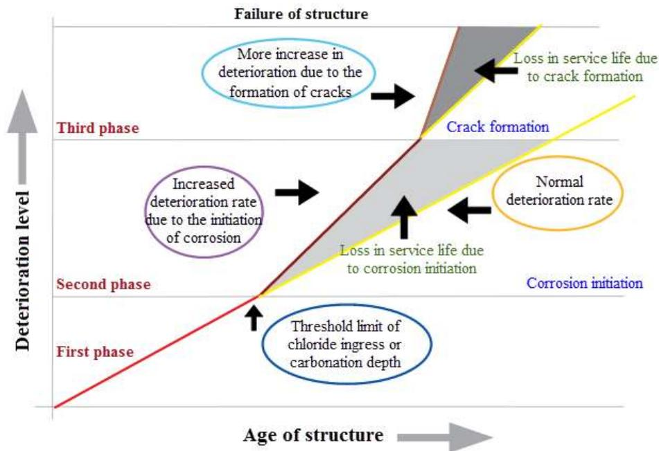
Fig. 2. Main events related to the service life of concrete structures [11].
