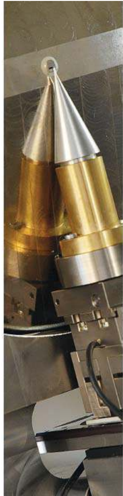
Figure 4: Specimen holder and object manipulation stage of the NanoXCT demonstrator
