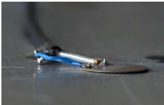
*Figure 1 – partially debonded PWAS*
