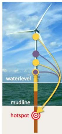
Figure 1 : Instrumentation of the monopile OWT at the Belwind farm. In yellow are the installed accelerometers and in purple the attached strain gauges. The upper levels of acceleration and strain are used in order to predict the strains at the lower levels.
