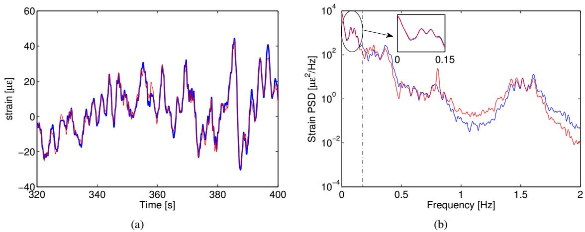
Figure 5 : Strain response on a wavy day. (a) Time domain response. In blue are the measured strain responses and in red are the predicted strains with the proposed multi-band virtual sensing scheme, (b) Power spectral density (PSD) of the measured (blue) and predicted (red) signals.
