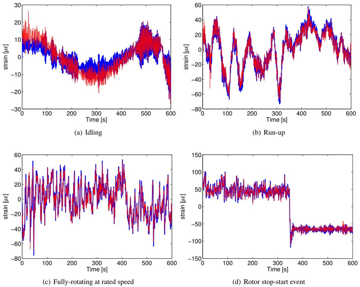
Figure 4 : (a-c) Normal operating conditions, (d) rotor stop-start extreme event. Ten minute strain time histories; In blue are the measured strain responses and in red are the predicted strains with the proposed multi-band virtual sensing scheme
