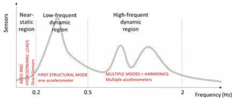
Figure 3 : Multi-band virtual sensing scheme
