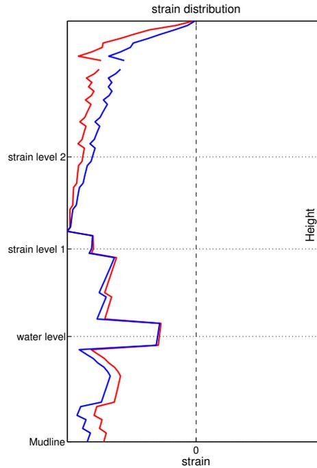
Figure 2 : Static strain distribution (red) and 1<sup>st</sup> FA/SS strain mode shape (blue) from mudline to tower top level
