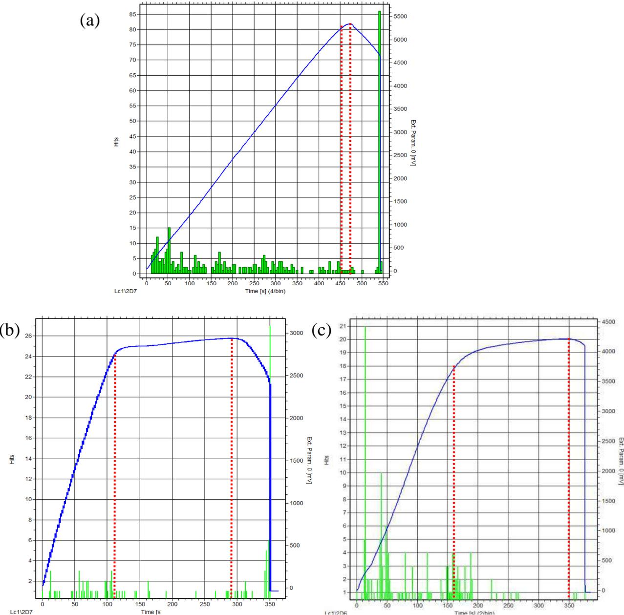
Figure 4: Stress and cumulative counts/hits versus time for displacement rate = 0.1 mm/min; (a) steel, (b) aluminium, and (c) brass
