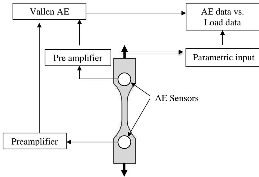
Figure 2: Schematic of experimental set-up
