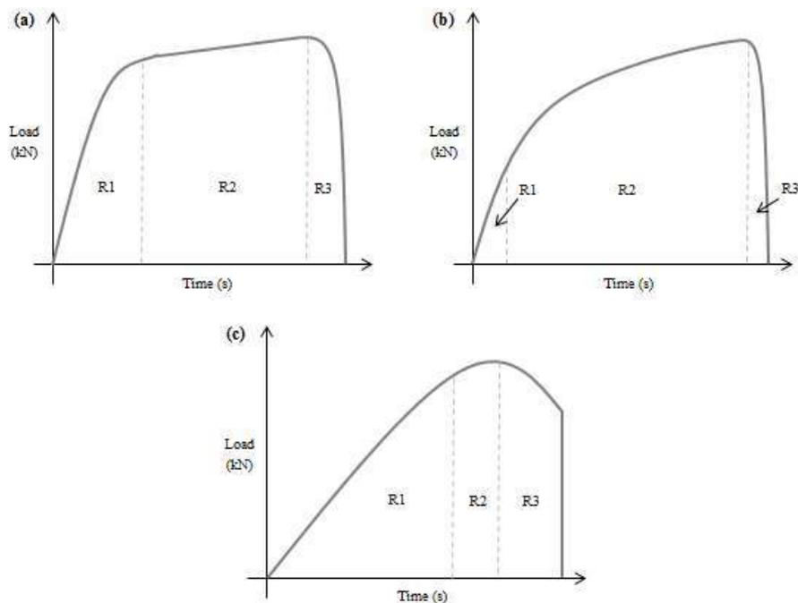
Figure 3: Metallic tensile loading regions (a) aluminium; (b) brass; (c) steel
