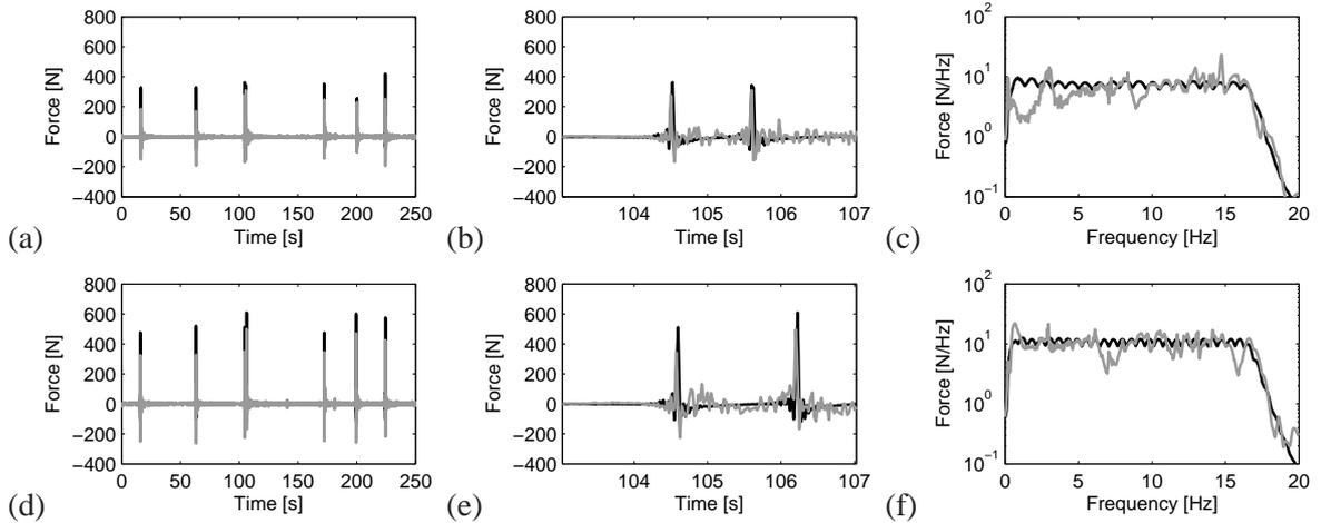
Figure 4 : Time history (left), detail of the time history (middle), and averaged amplitude of the narrow band frequency spectrum (right) of the hammer forces applied at node 27 ((a) – (c)) and node 48 ((d) – (f)). The measured force signals are shown in black, the identified force signals are shown in gray.
