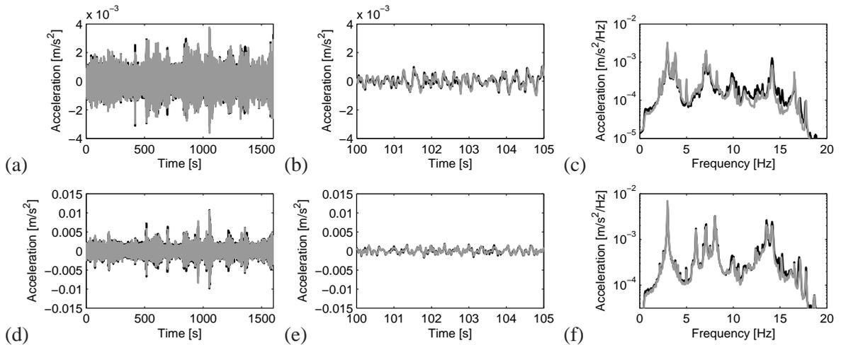
Figure 5 : Time history (left), detail of the time history (middle), and averaged amplitude of the narrow band frequency spectrum (right) of the lateral ((a) – (c)) and vertical ((d) – (f)) acceleration at node 7. The measured accelerations are shown in black, the estimated accelerations are shown in gray.
