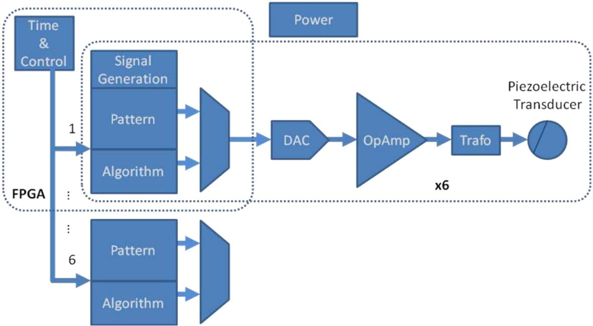
Figure 4. Block diagram of the generation part of the G6AC board.
