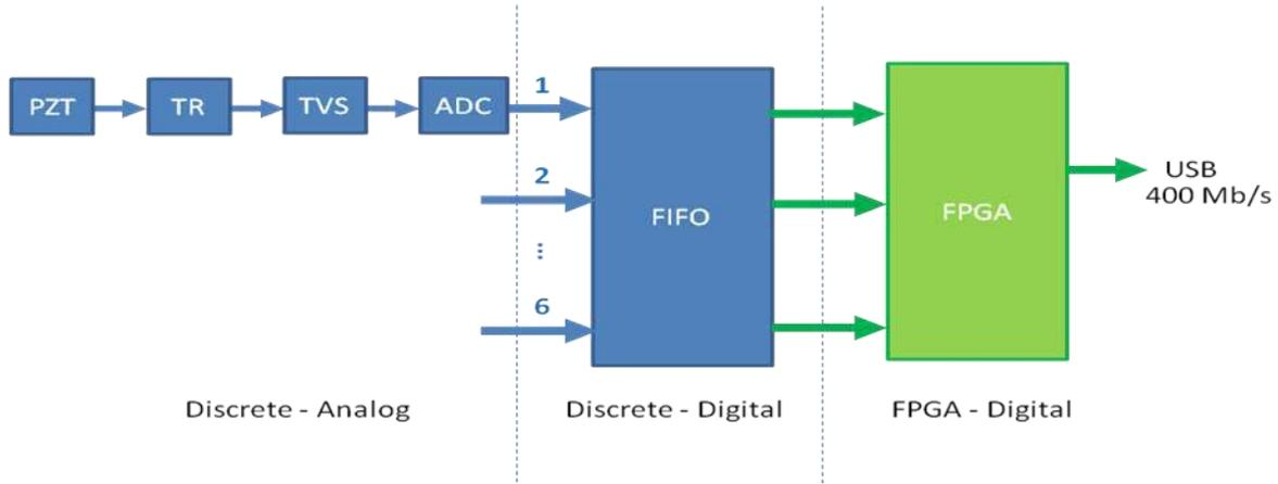
Figure 5. Block diagram of the acquisition part of the G6AC board.
