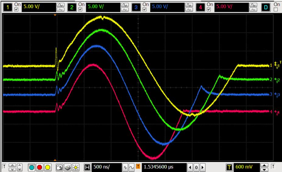
Figure 7. Voltage measurement of four of the output channels in SHMUS. All the signals have different period and frequency.
