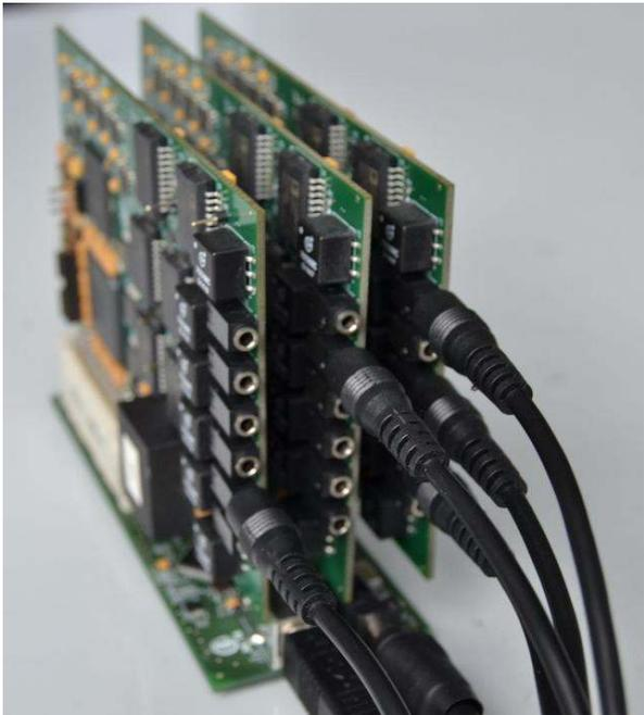
Figure 2. Actual SHMUS prototype that includes the connection of three GA6C boards.
