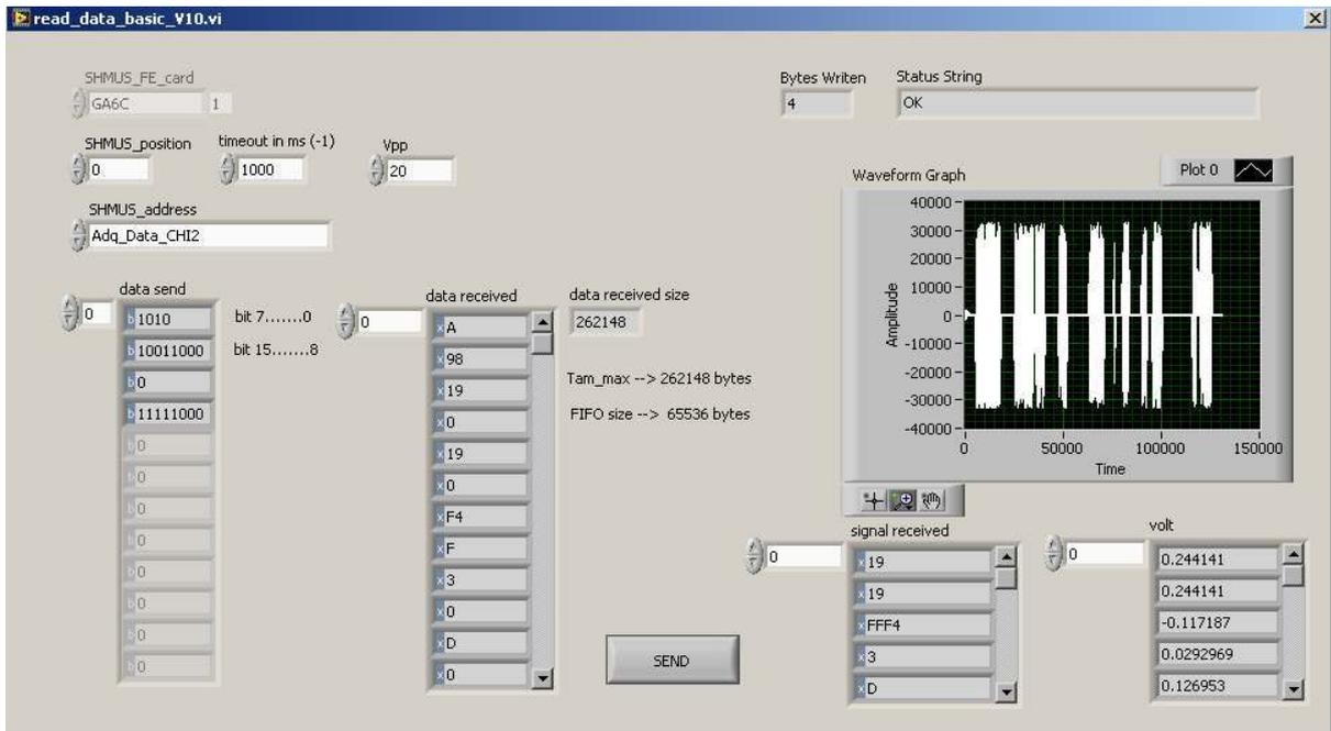
Figure 9. Software for the acquisition control in SHMUS.
