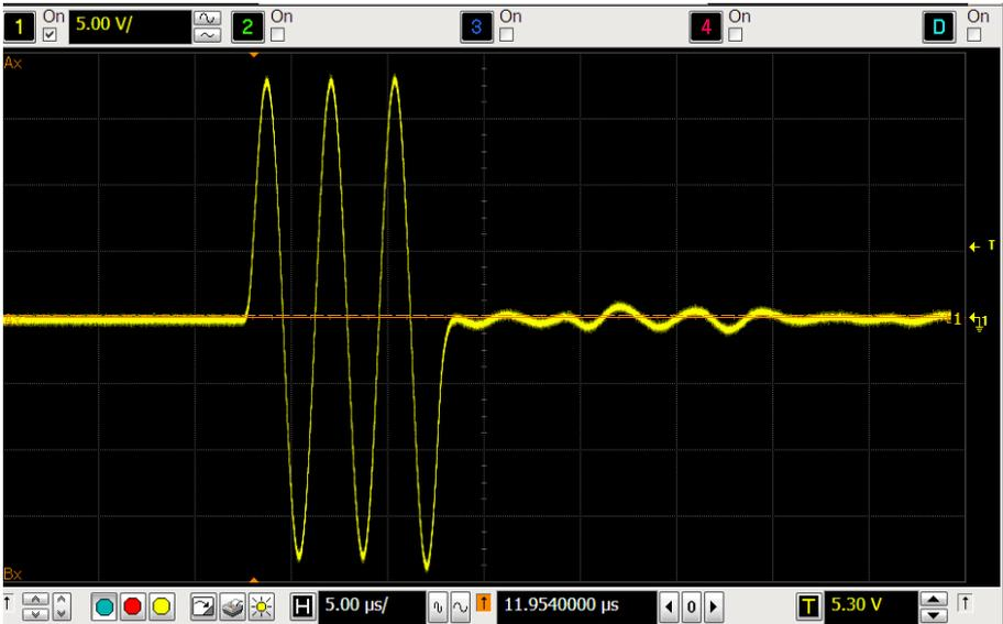
Figure 6. Example of output signal in SHMUS when applied to a piezoelectric load.
