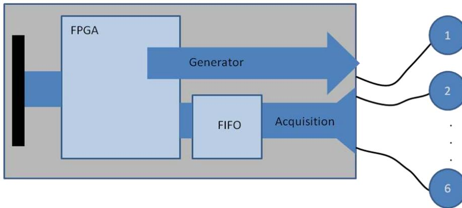
Figure 3. Block diagram of the GA6C board.
