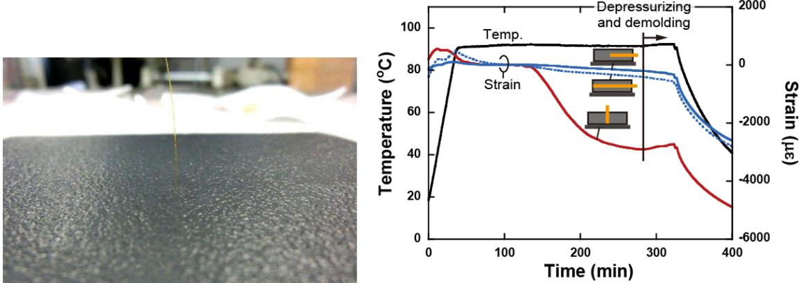
Figure 8: (Left) Surface of specimen with through-thickness sensor. Optical fiber is extending perpendicularly from surface. (Right) Transversely anisotropic shrinkage of unidirectional carbon/epoxy induced due to tool-part interaction. Measurement under practical curing condition is possible with this approach [9].
