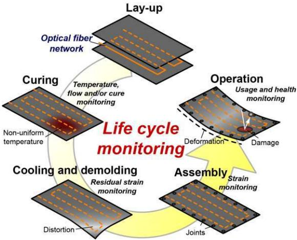
Figure 1: Life cycle monitoring of composite structures [2].
