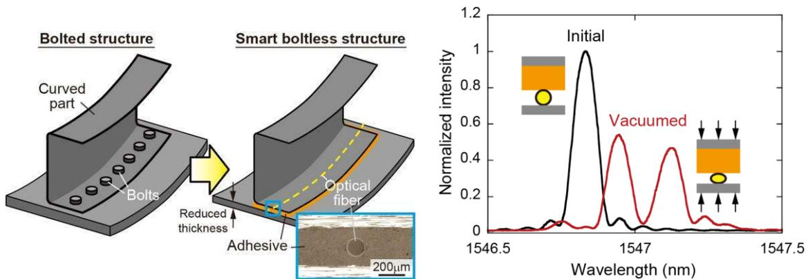
Figure 7: (Left) Smart boltless structure with embedded optical fiber sensor. Without bolts, component thickness can be reduced and more efficient load path is possible. (Right) FBG spectrum just after vacuuming. Using this response, manufacturing workers can immediately identify areas with lack of bonding pressure [8].
