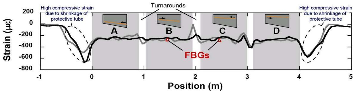
Figure 3: Thermal residual strain obtained from two lines embedded in the same position. Result agreed well with FBG measurement, validating measurement accuracy [2].
