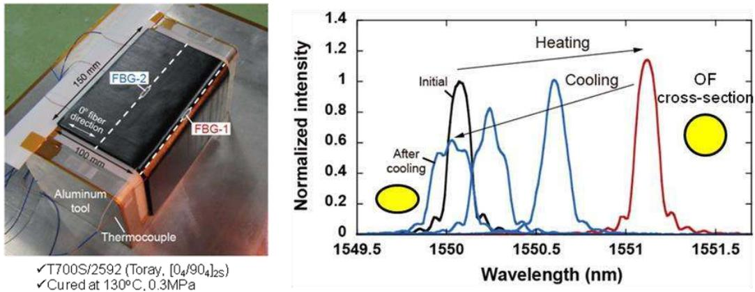
Figure 4: Process monitoring of L-shaped corner part. Through-thickness strain was continuously monitored using birefringence effect of FBG sensor [5].
