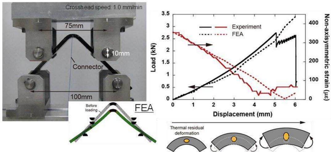
Figure 5: Through-thickness strain monitoring during four-point bending test of L-shaped corner part [5].
