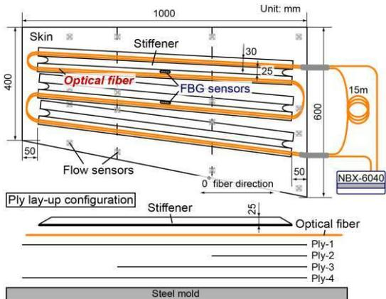
Figure 2: CFRP panel for demonstration fabricated through VaRTM process [2].
