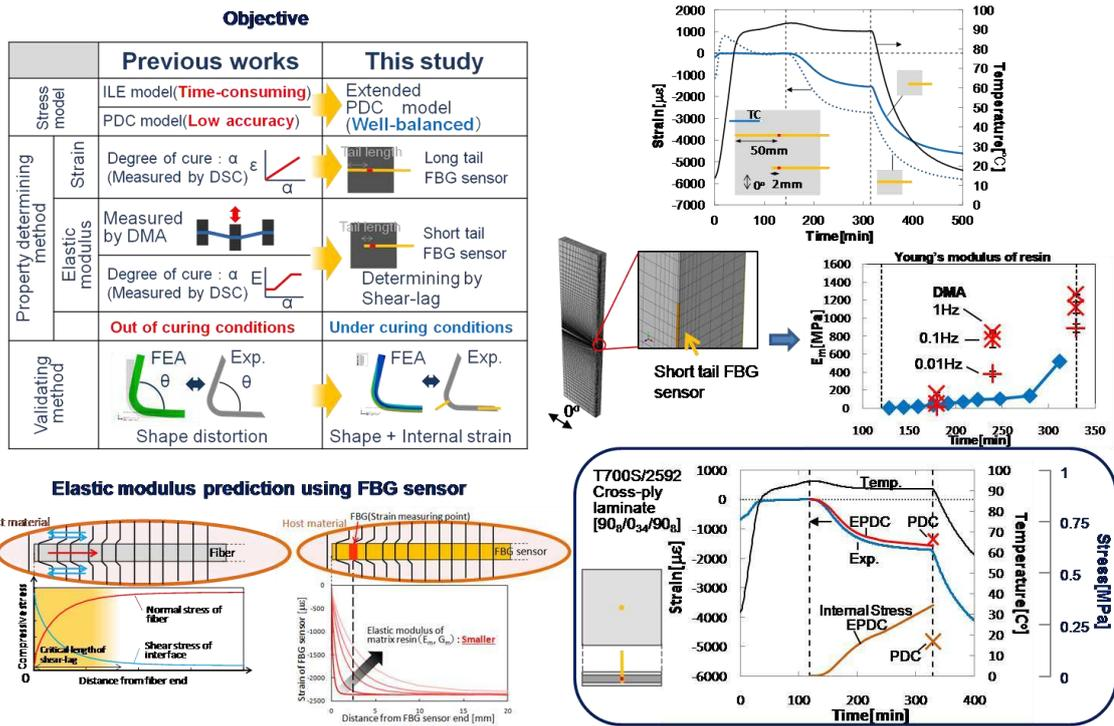
Figure 9: Composite cure simulation scheme fully integrating the fiber-optic-based measurement [10].
