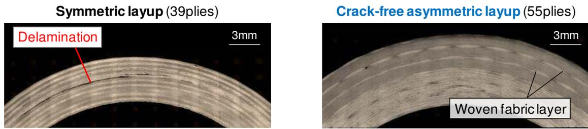
Figure 6: Cross-section of thick-walled CFRP pipes. No delamination failure was observed in proposed asymmetric lay-up. Stress reduction effect was validated using fiber-optic-based monitoring system [7].
