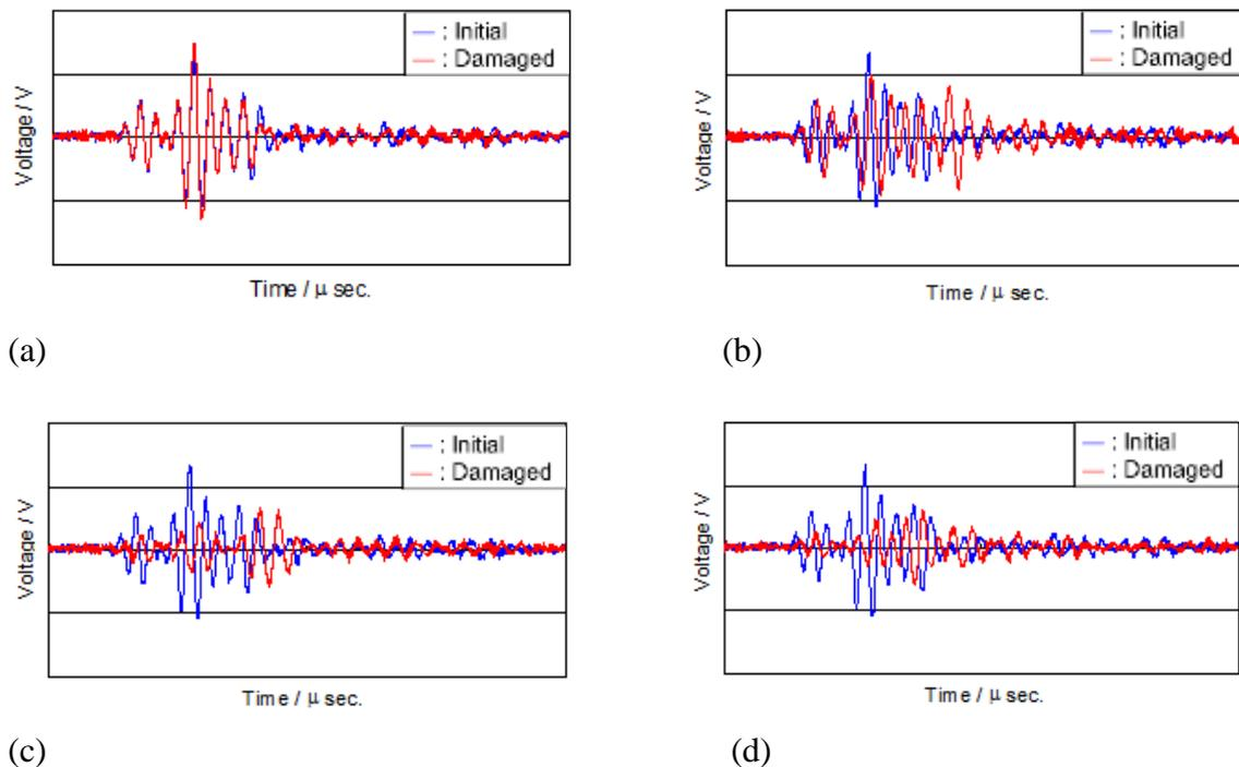
Figure 10 Measured Lamb waves at “hot-spot” with BVID.
