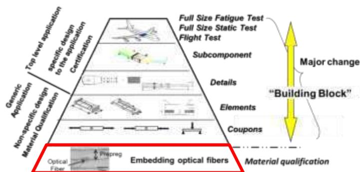
Figure 4 Building Block Approach concept.
