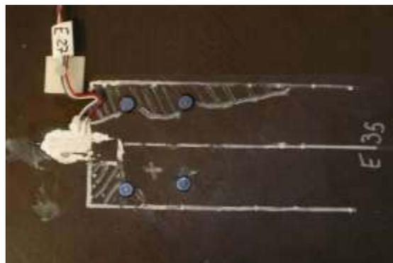
Figure 12 Overview of damage condition near the "hot-spot" after applying load 290 kN.
