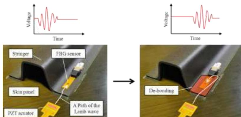
Figure 2 Principle of the "Time delay" analysis method.
