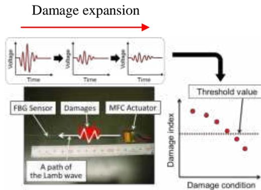
Figure 3 Principle of the "Waveform change" analysis method.
