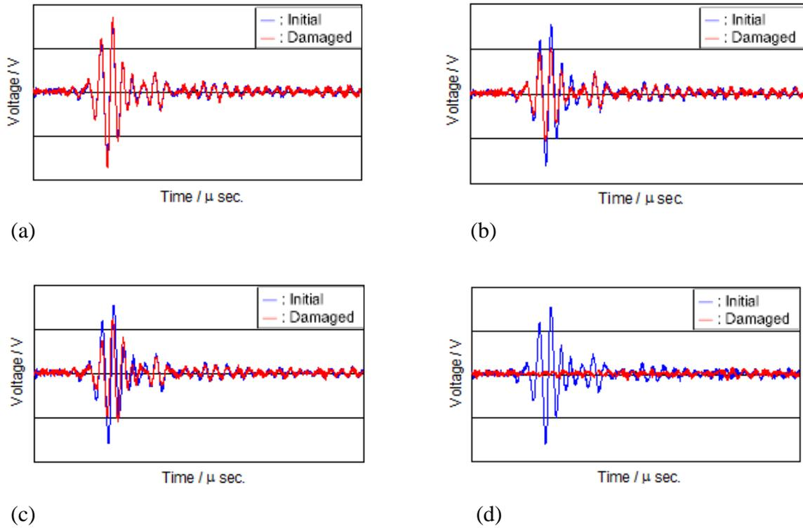
Figure 11 Measured Lamb waves at “hot-spot” with artificial defect.
