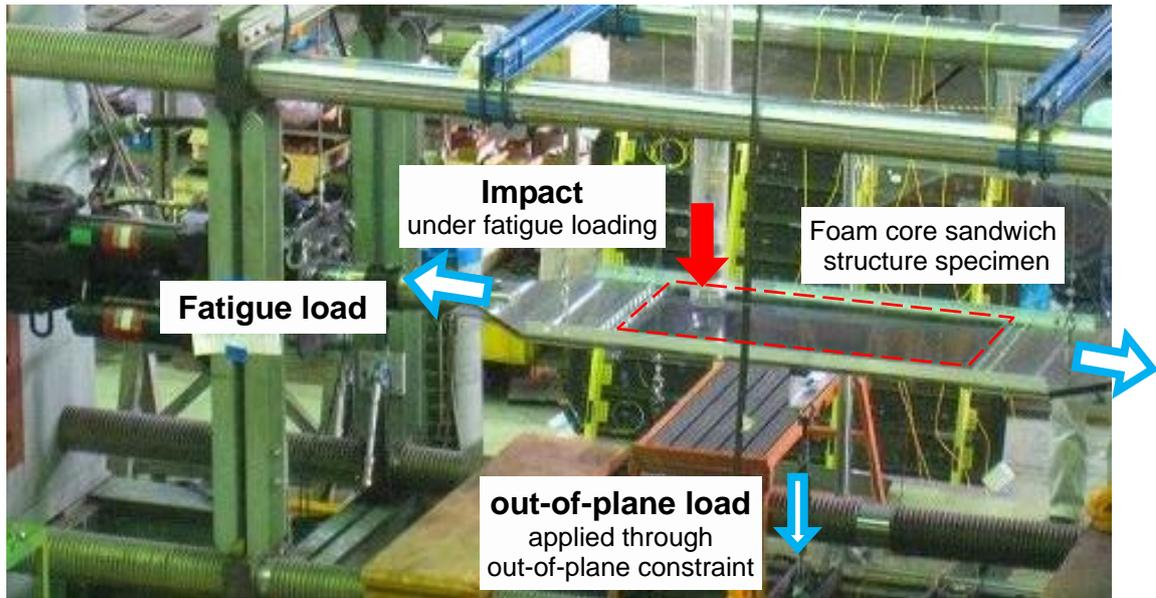
Figure 11: Impact test setup
