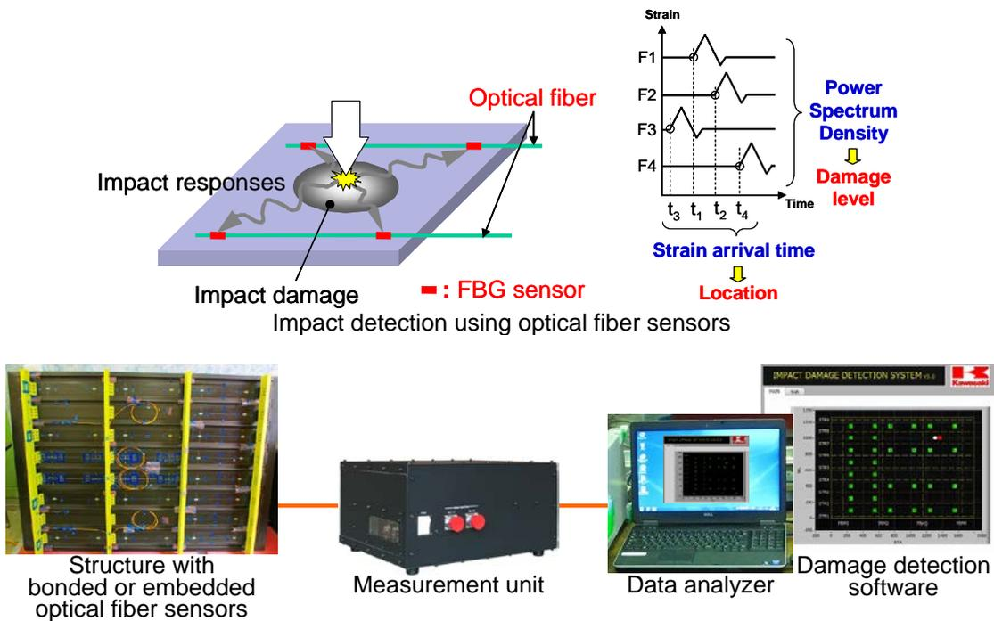
Figure 1: Impact Damage Detection system
