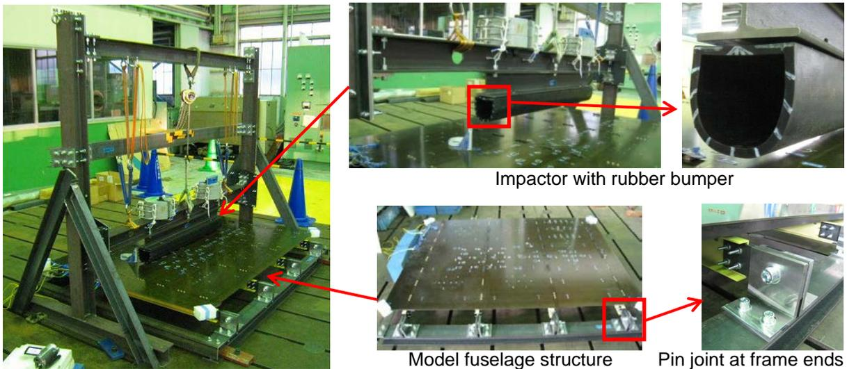
Figure 2: BOI test setup
