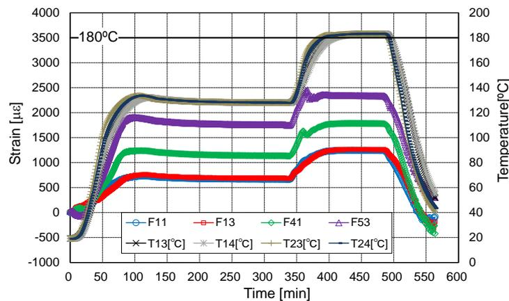
Figure 10: Example of the cure process monitoring
