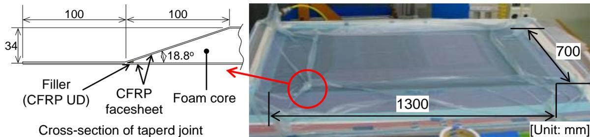
Figure 9: Foam core sandwich panel before cure
