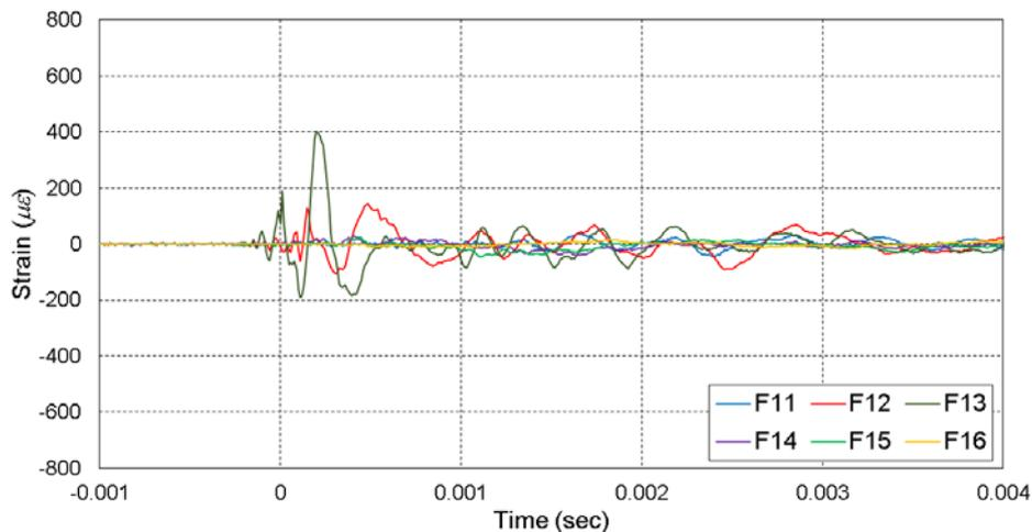
Figure 7: Example of the impact strain response measurement (at impact location I41, below the BVID level)
