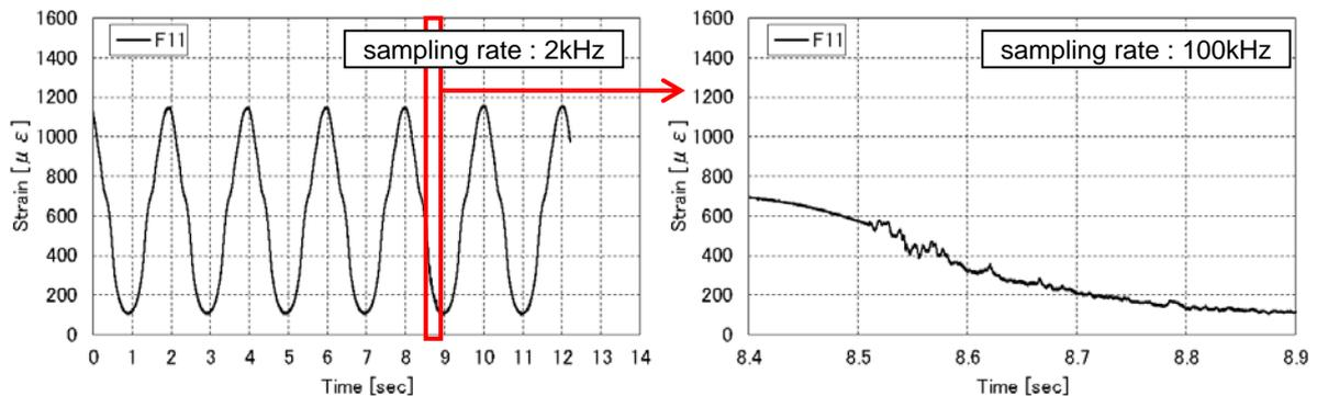
Figure 12: Example of the impact response during fatigue loading
