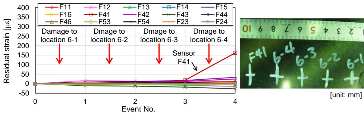
Figure 13: Example of the crack propagation monitoring test
