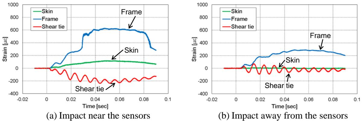
Figure3: Example of the BOI strain response
