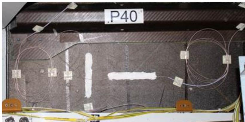
Figure 6: Example of the sensing line installation
