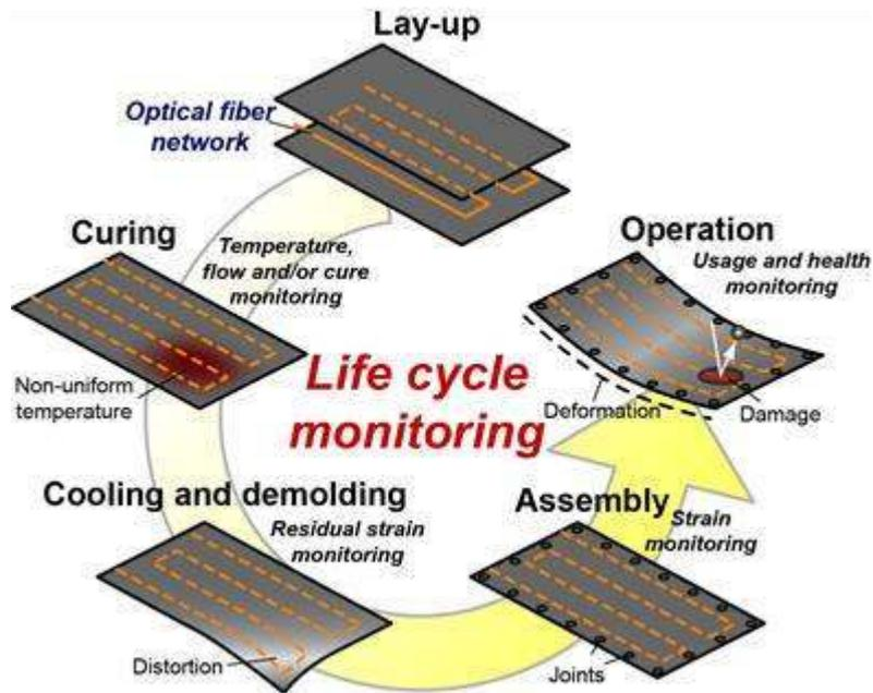
Figure 3: Concept of Life cycle monitoring. [3]
