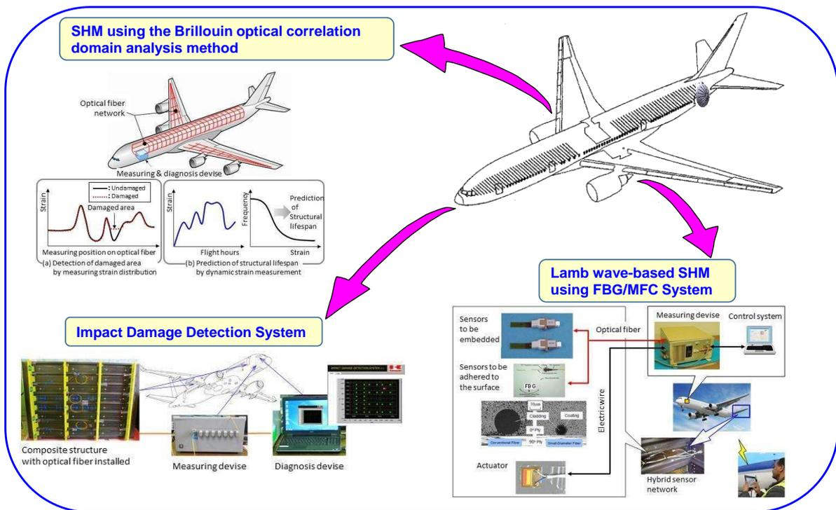
Figure 2: Three SHM systems in the METI Project.
