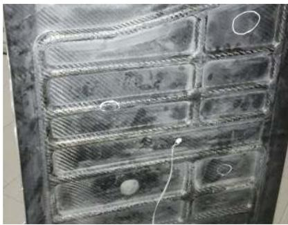
Figure 11: CFRP aerospace panel with stiffeners.
