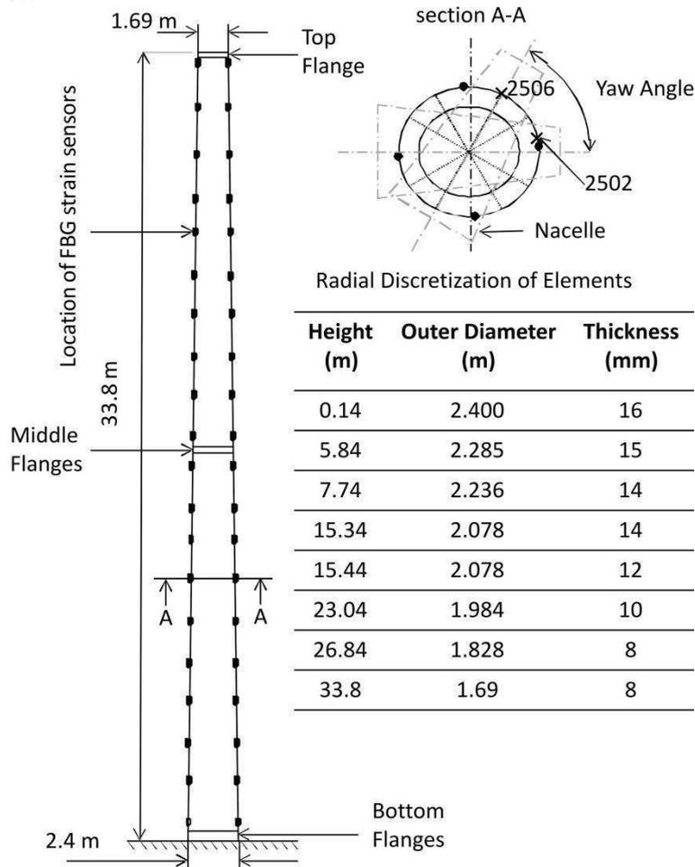
Figure 7: FE modelling details of Nordtank NTK 500/41 wind turbine [8].
