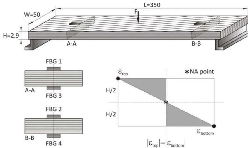
Figure 3: Experimental setup for composite beam.
