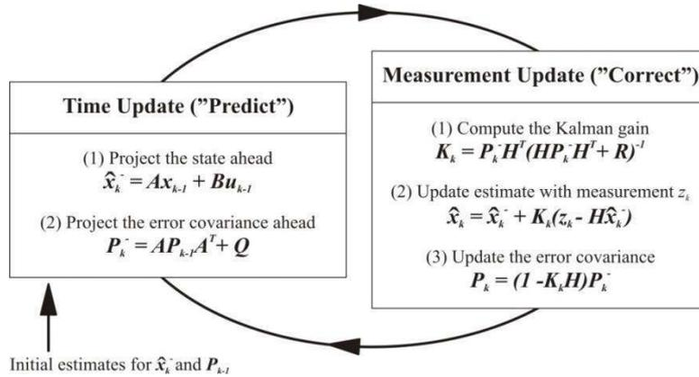
Figure 2: Flow chart for the implementation of the KF [11].
