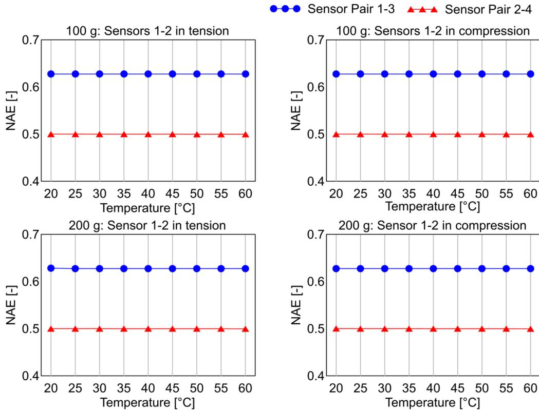
Figure 6: Estimated NA with temperature compensation under static loading of 100g and 200g under varying temperature conditions
