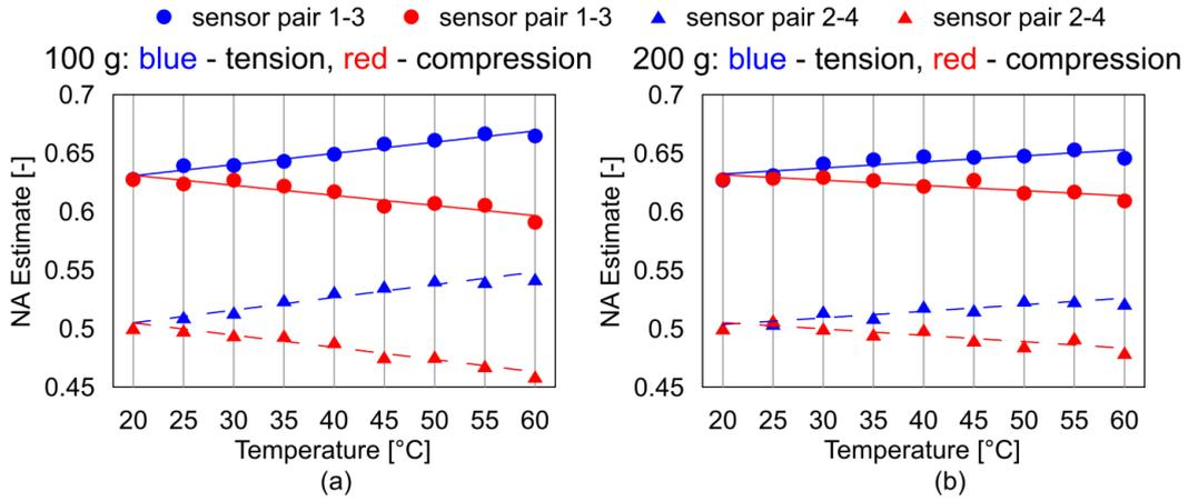
Figure 5: Estimated NA without temperature compensation under varying temperature conditions. (a) 100g static loading (b) 200g static loading
