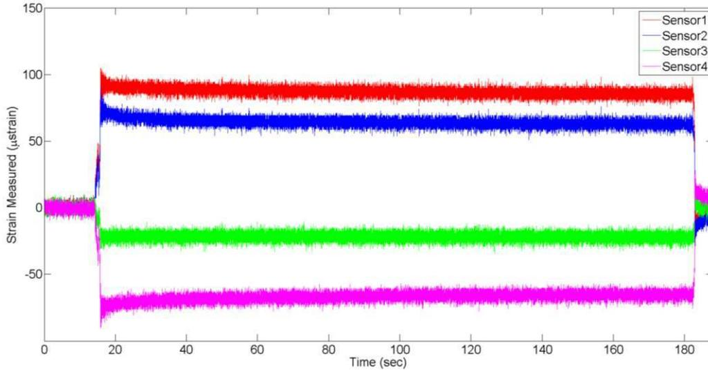
Figure 4: Measured strain in composite beam.
