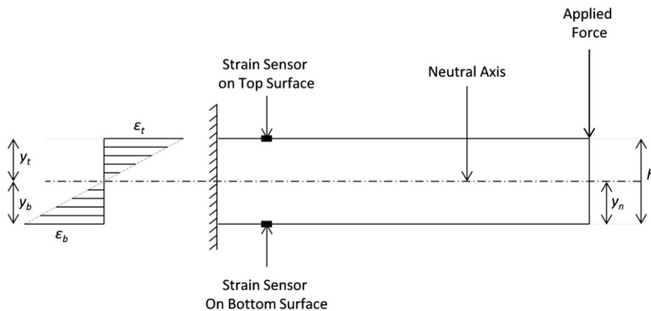
Figure 1: Flexural strain distribution over the beam cross section.
