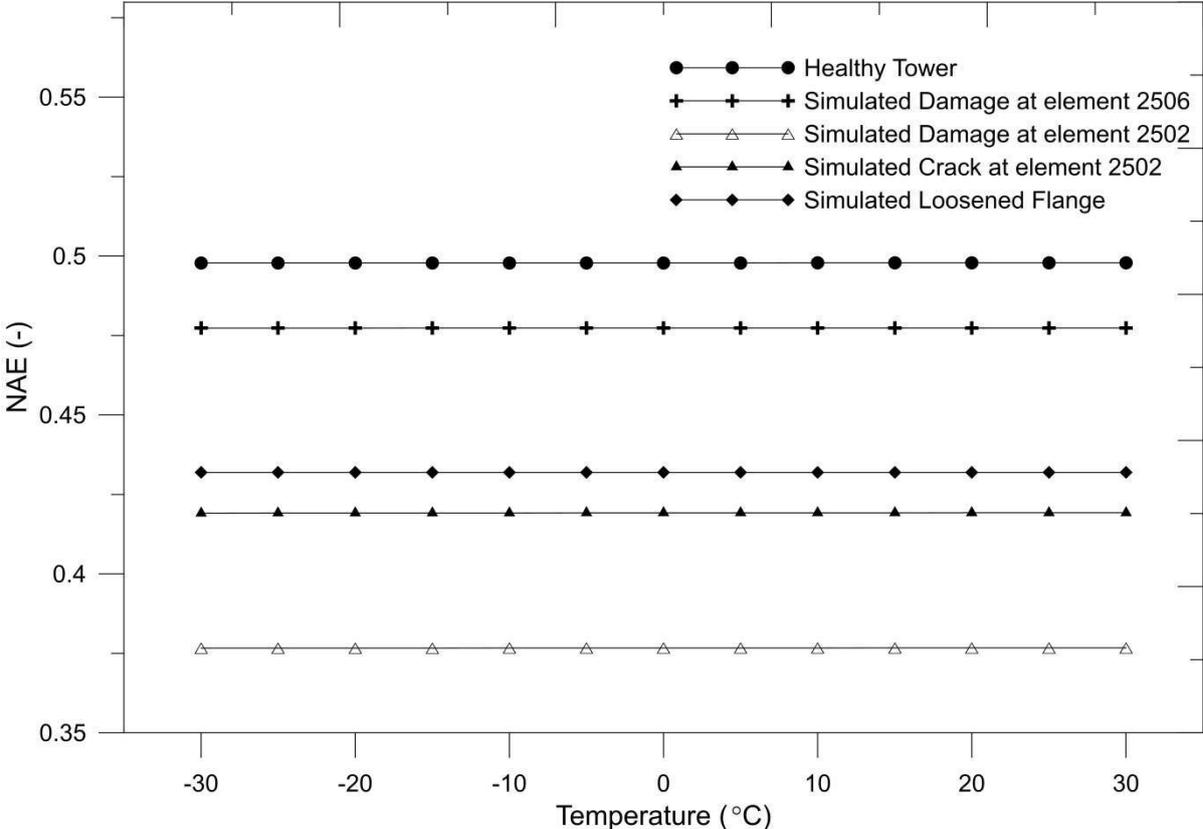
Figure 8: Change in NAE position with ambient temperature.
