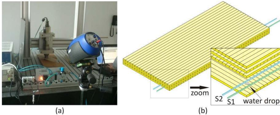
Figure 1. (a) The set up of vibrothermography with sample, (b) schema of sample with zoom on its internal structure, where S1 and S2 are the fibre optics.
