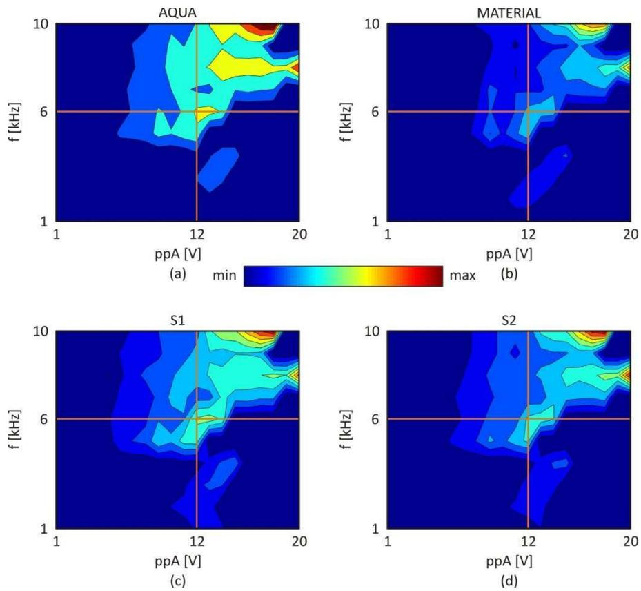
Figure 4. Maps showing relation between frequency and peak-to-peak amplitude for selected areas.
