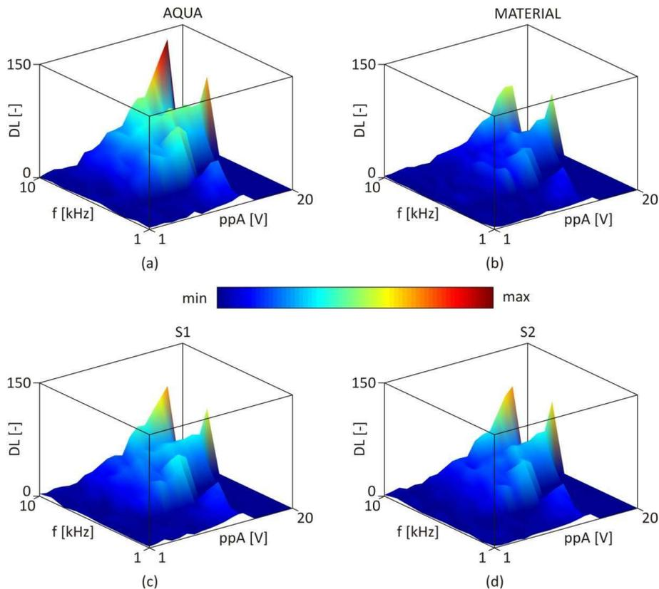
Figure 3. The temperature distribution in function of frequency and peak-to-peak amplitude for selected areas.
