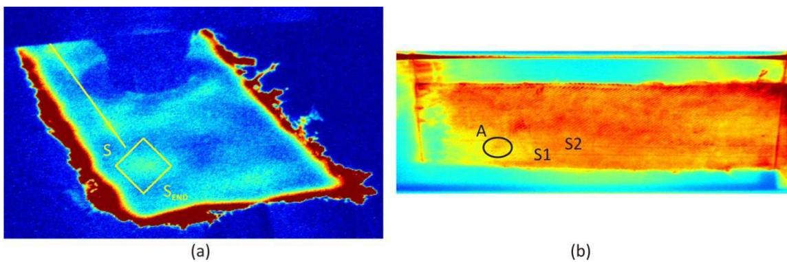
Figure 10. Thermogram of (a) a sample with broken fibre optic (vibrothermography) (b) a sample with fibre optics and drop of water (impulse thermography).
