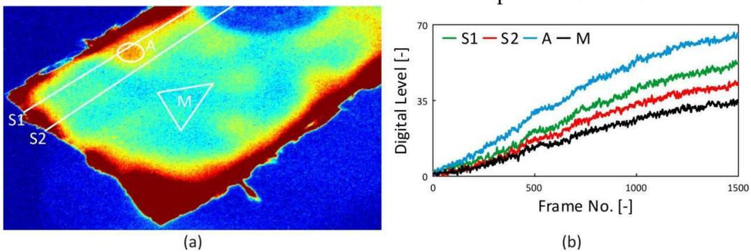
Figure 2. (a) An example of thermogram (6 kHz and 12V), (b) an average timing-graph for chosen area.
