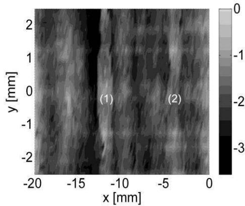
Figure 11. Map originated from deconvolution method presenting location of embedded fibre optics in sample (Figure 2 (a)); (1) and (2) embedded fibres.
