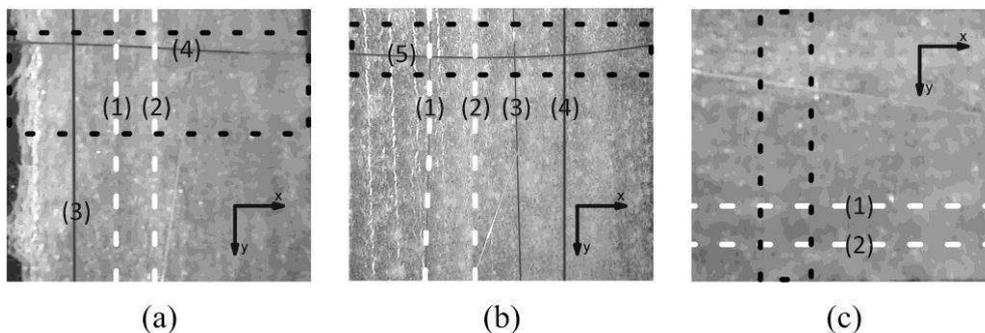
Figure 2. Three (a), (b), (c) GFRP samples with fibre optics: embedded into material structure (1), (2) and lying on the samples' surfaces (3)–(5).
