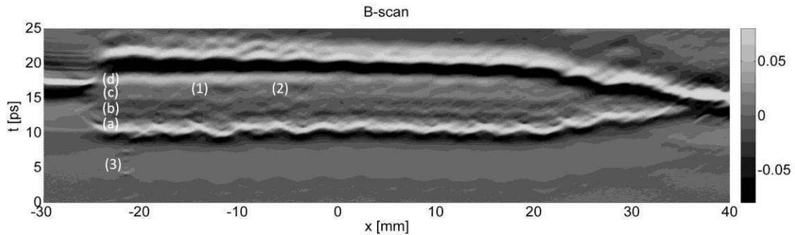
Figure 3. B-scan from the rough side of the sample; (a)–(d) composite layers; (1) and (2) – embedded fibres, (3) fibre lying on the sample surface.
