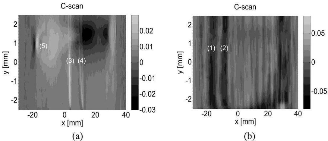
Figure 7. C-scans presenting (a) fibre optics lying on the sample surface and (b) embedded in composite material; (1) and (2) – embedded fibres, (3)–(5) fibres lying on the sample surface.
