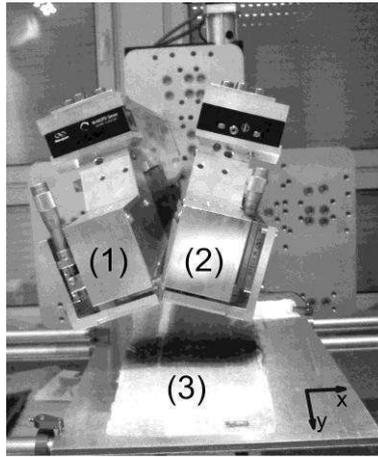
Figure 1. THz spectrometer in the reflection mode: (1) – emitting head, (2) – receiving head, (3) GFRP sample on a metal table.
