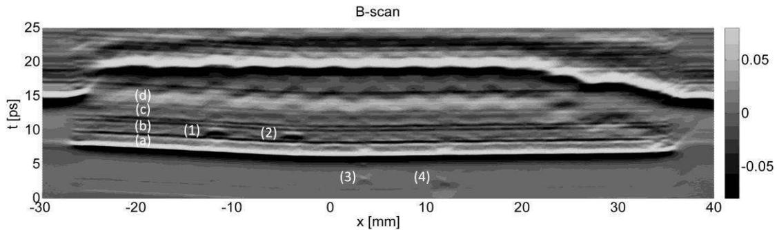
Figure 5. B-scan for the smooth side of the sample; (a)–(d) composite layers; (1) and (2) – embedded fibres, (3) and (4) fibres lying on the sample surface.
