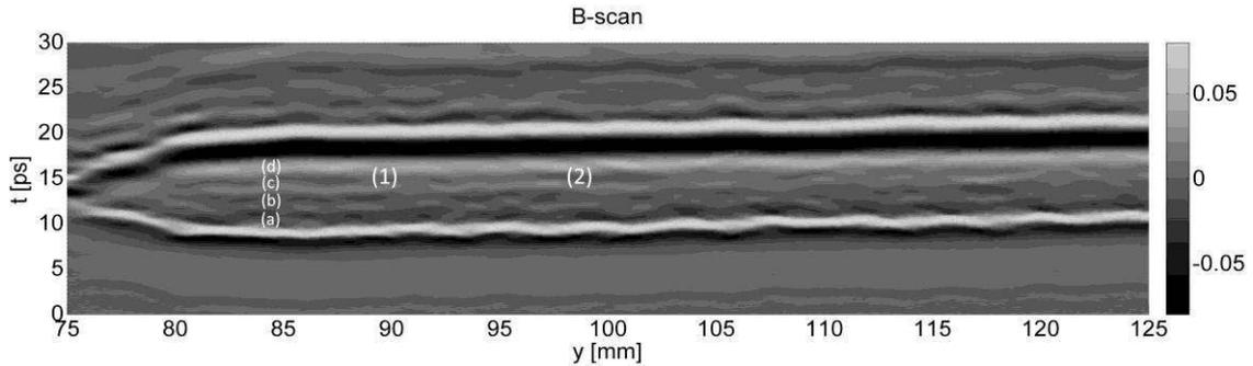
Figure 8. B-scan for the sample with FBG sensors lying parallel to the x direction; (a)–(d) composite layers; (1) and (2) – embedded fibres.
