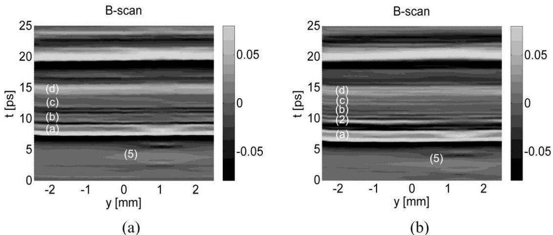
Figure 6. B-scans presenting material structure: (a) without embedded fibre, (b) with embedded fibre; (a)–(d) composite layers; (2) – embedded fibre, (5) fibre lying on the sample surface.
