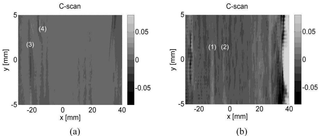
Figure 4. C-scans presenting (a) fibre optics lying on the sample surface and (b) embedded in composite material; (1) and (2) – embedded fibres, (3) and (4) fibres lying on the sample surface.
