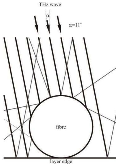
Figure 10. Schema of THz wave interaction with circular fibre parallel to the y axis of the THz unit.
