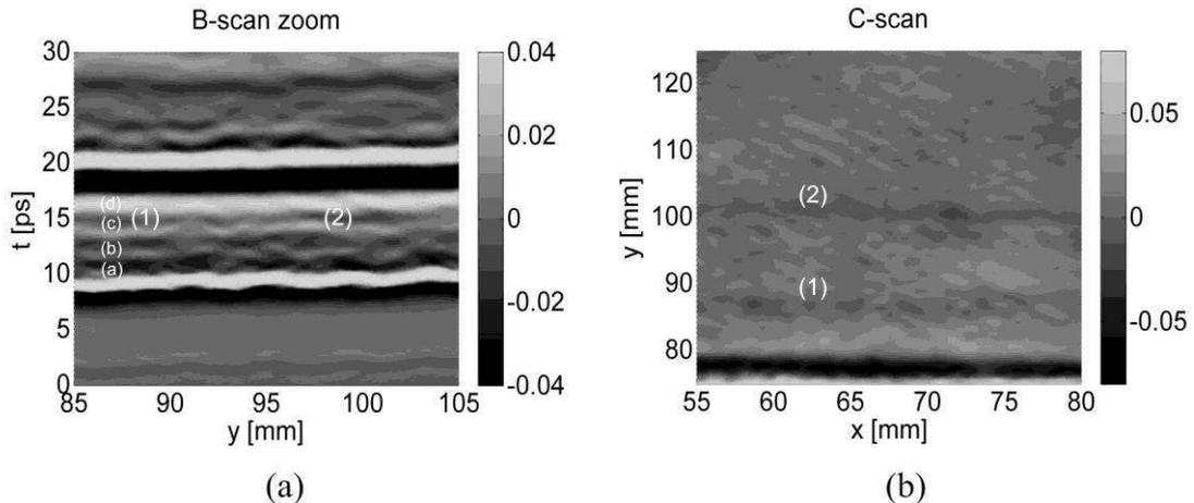
Figure 9. Sample with optic fibres lying parallel to the x direction of the THz unit: (a) B-scan with a part of the sample with embedded optic fibres, (b) C-scan presenting fibres embedded in composite material; (a)–(d) composite layers; (1) and (2) embedded fibres.
