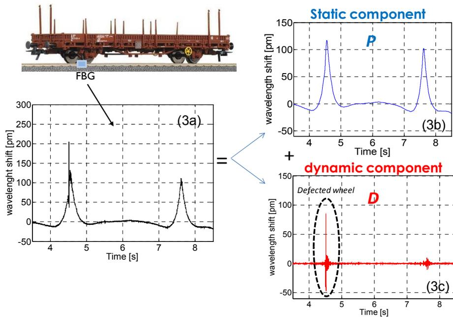
Figure 3: Raw FBG sensor signal (3a), static (3b) and dynamic (3c) component.
