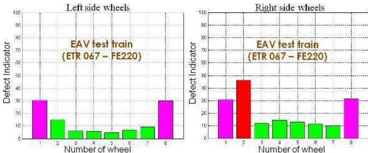
Scanner laser measurements (EAV) and WLD system's outputs
