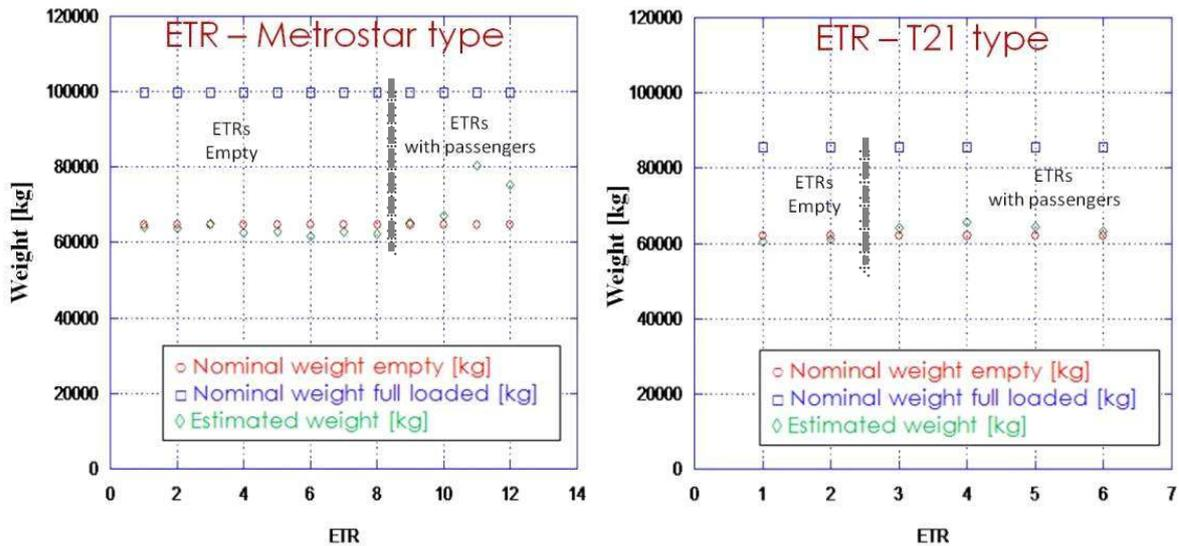
Figure 10: Weight tests on ETR in normal operation (Empty ETRs or ETRs with passengers)
