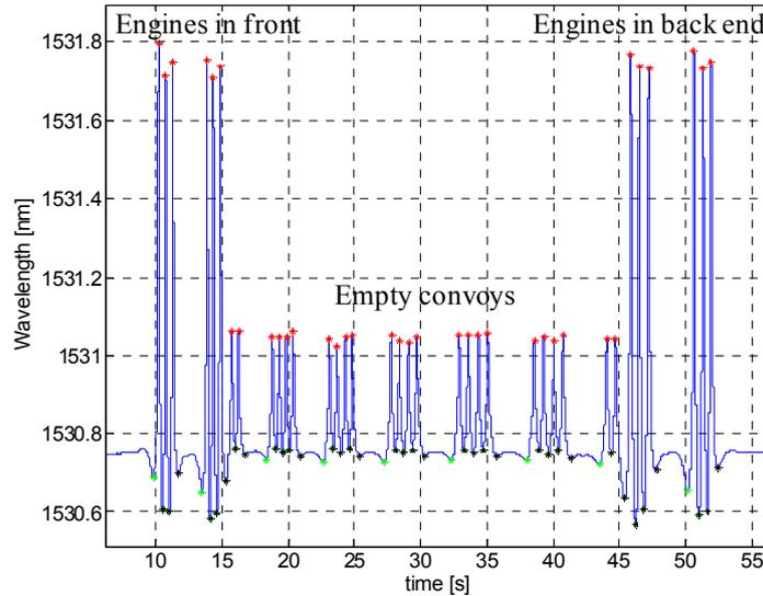
Figure 2: Typical response returned by a FBG clamped to the rail during a transit of a train.
