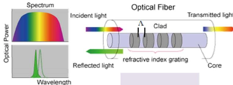
Figure 1: Incident, transmitted and reflected light in a Fiber Bragg Grating.
