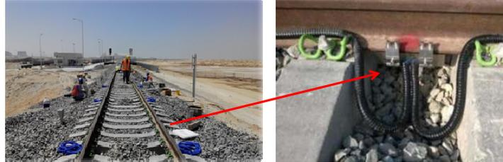
Figure 7: WIM system prototype and WIM sensor along Abu Dhabi railway
