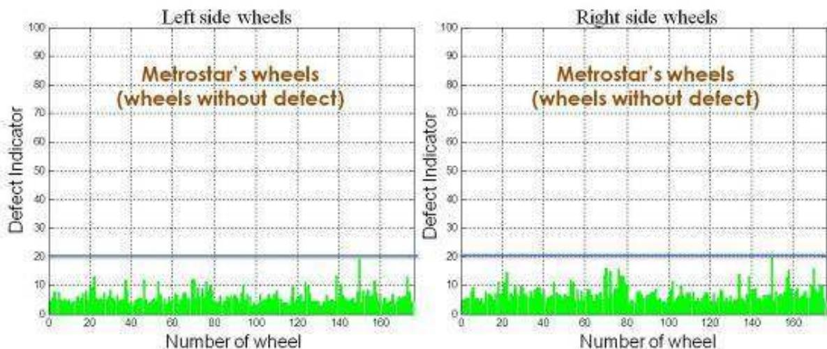
Figure 12: threshold value for new wheels
