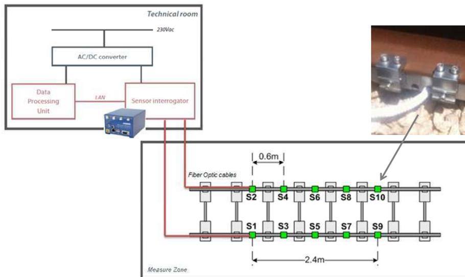
Figure 4: TWBCS typical installation layout
