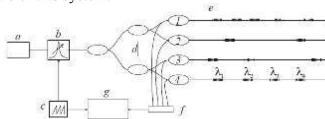
Figure 6: Interrogator scheme: a) optical source, b) filter scan, c) sweep generator, d) splitter, e) FBG, f) photo detectors, g) processor.
