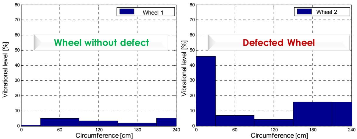
Figure 11: typical example of vibrational levels for defected wheel and for wheel whitout defect
