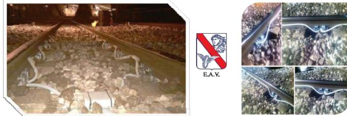
Figure 8: WIM - WFD system prototype along the rail of Garibaldi central station
