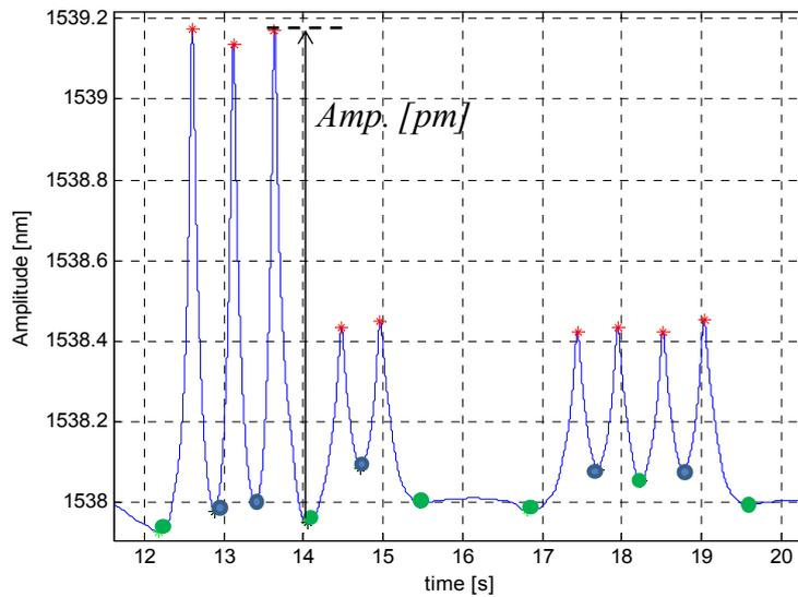
Figure 9: FBG response and wavelength shift related to the weight force
