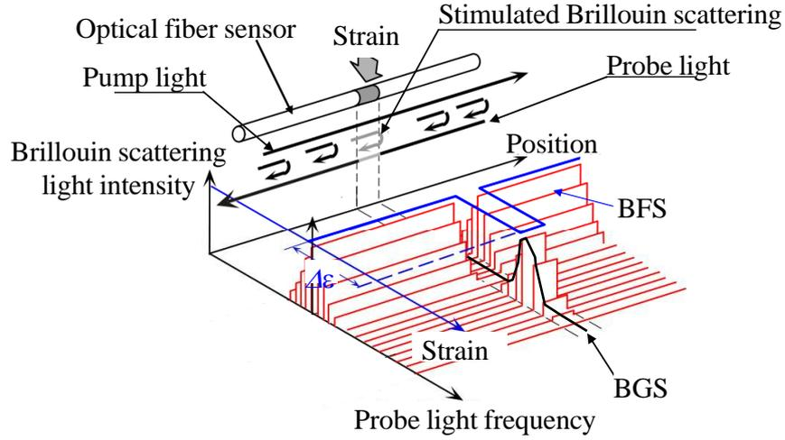
Figure 3: BOCDA measurement principle
