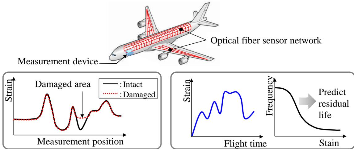
(a) Damage detection by distributed sensing (b) Fatigue life prediction by dynamic sensing
