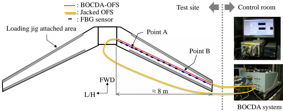
Figure 4: Overview of the full scale horizontal tail plane
