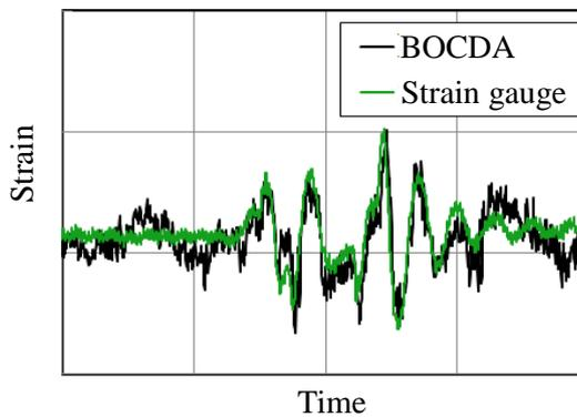
Figure 9: Dynamic strain measurement result
