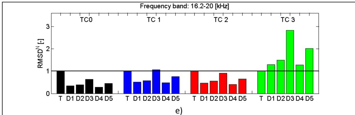
Figure 4: Influence of temperature compensation on RMSD index values for different sample state, for different frequency sub-bands: a) 1–4.8 kHz, b) 4.8–8.6 kHz, c) 8.6–12.4 kHz, d) 12.4–16.2 kHz, e) 16.2–20 kHz.
