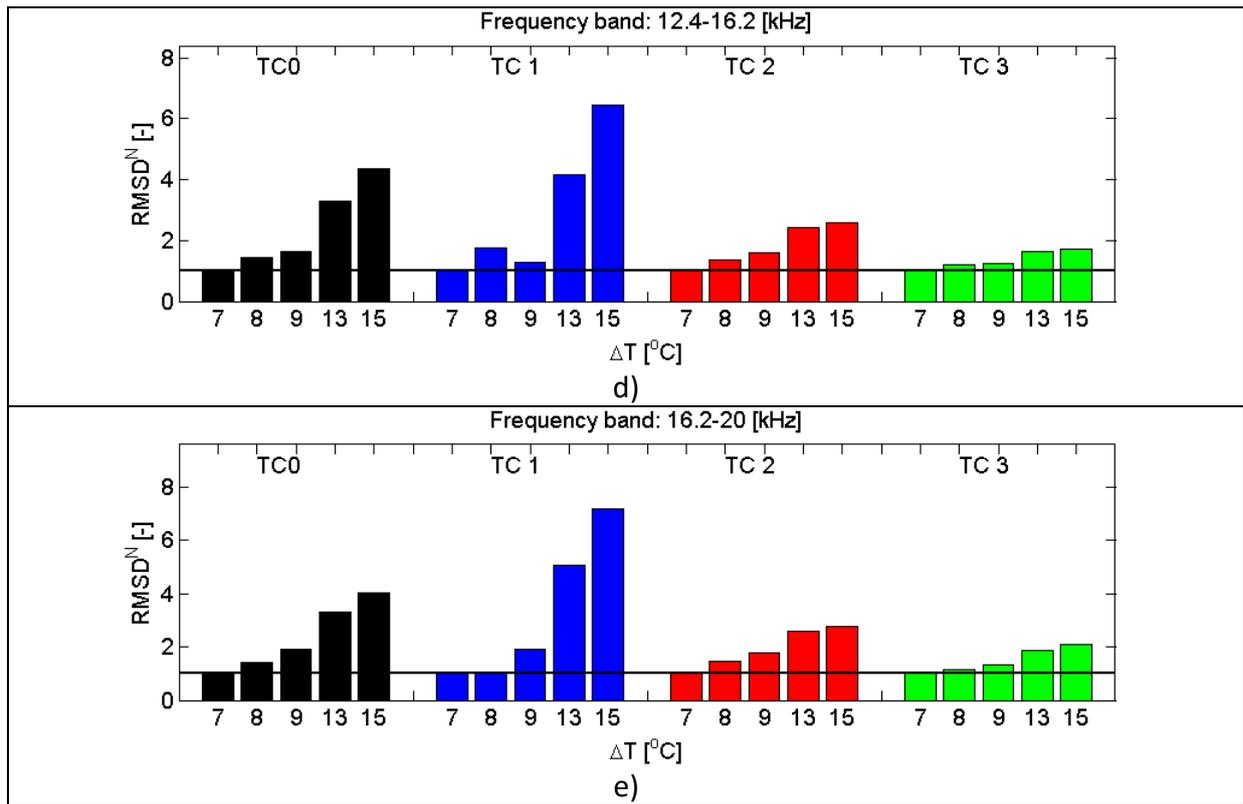
Figure 3: Influence of temperature compensation on RMSD index for different frequency subbands: a) 1–4.8 kHz, b) 4.8–8.6 kHz, c) 8.6–12.4 kHz, d) 12.4–16.2 kHz, e) 16.2–20 kHz.
