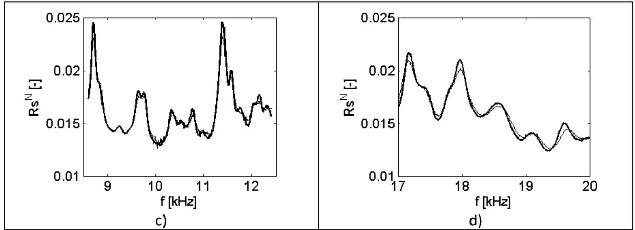
Figure 2: Results of temperature compensation (vertical shift) using normalization with RMS value, frequency range: a) 1–4 kHz, b) 5–8 kHz, c) 8.5 –12.5 kHz, d) 17–20 kHz
