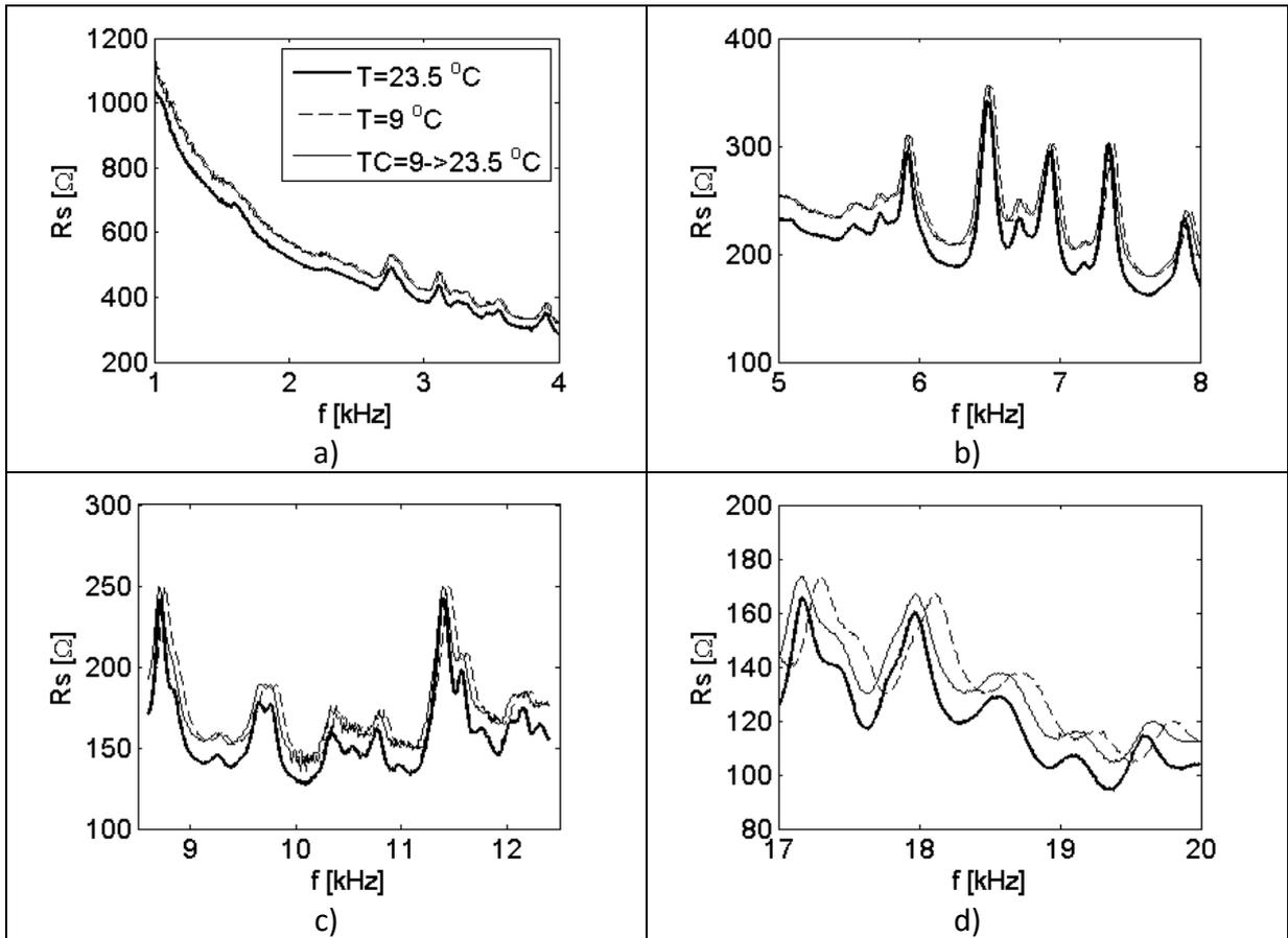
Figure 1: Results of temperature compensation (horizontal shift) using cross-correlation, frequency range: a) 1–4 kHz, b) 5–8 kHz, c) 8.5 –12.5 kHz, d) 17–20 kHz
