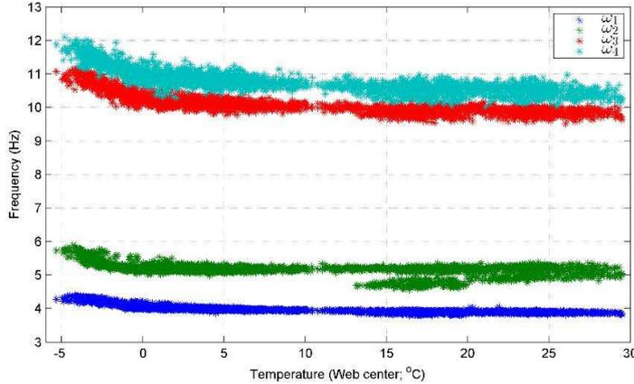
Figure 5. First four natural frequency estimates vs. temperature.
