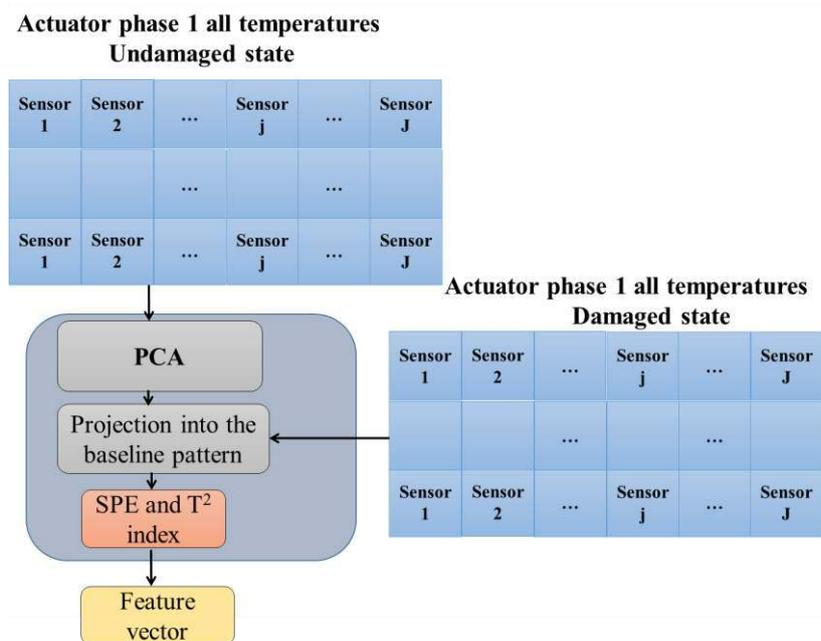
Figure 2: PCA modeling and damage detection index.
