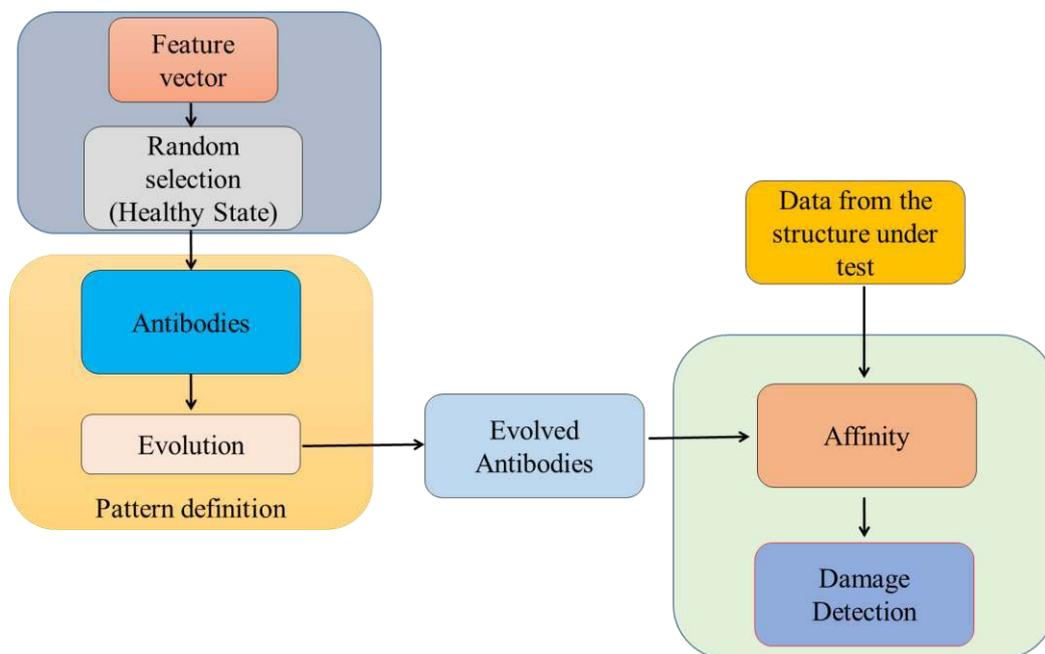
Figure 3: Damage detection process.
