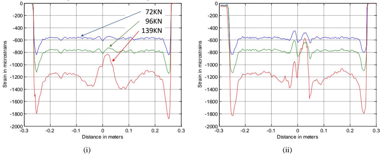
Figure 4: Static loading of the impacted panel: effect of impact on strain distribution along the stringer feet for (i) undamaged stringer and (ii) stringer with impact damage
