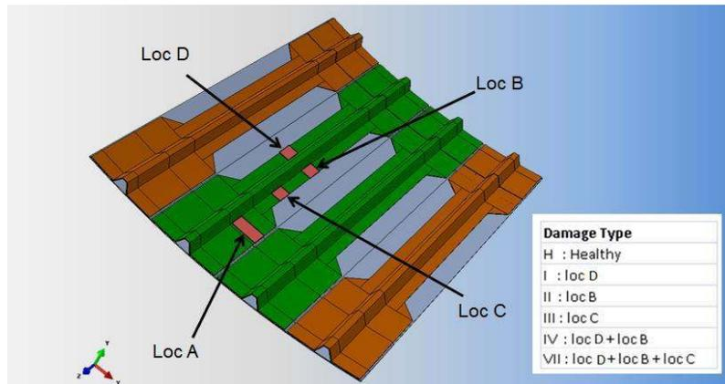
Figure 5. The FE model with the locations of the debondings, and all the simulated damage cases.
