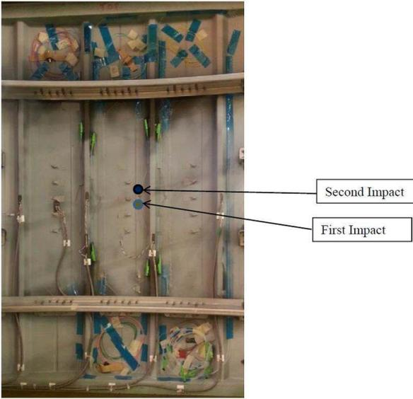
Figure 2: The stiffened skin panel, showing the locations of the barely visible impacts (The impact was performed on the outer side)
