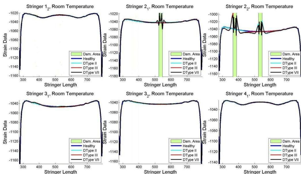
Figure 6. FEA strain data at room temperature, for all damage cases. Blue lines indicate healthy structure, while cyan, red and black lines indicate damage case II, III, and VII respectively. The green areas correspond to debonding locations.
