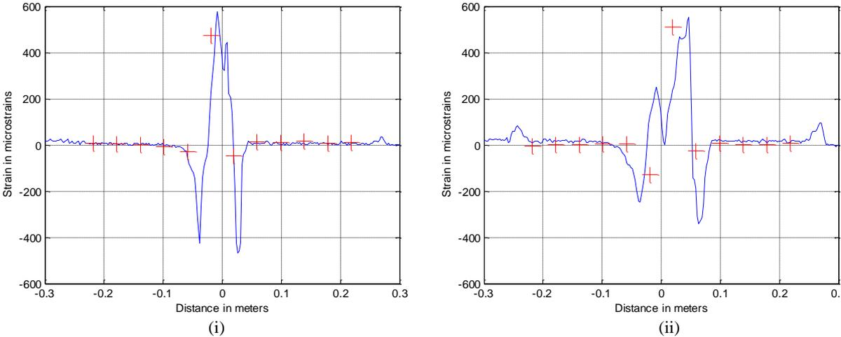
Figure 3: Impact test results. Rayleigh Backscattering distributed Strain Sensing (solid continuous line) and FBG point readings (+), measured after each impact test. The pre-impacts state was used as a reference. (i) First impact, (ii) second impact. The interrogator was Luna OBR4600 on courtesy loan from Luna Innovations Incorporated. The high speed FBG interrogator (20 kHz of sampling rate) is a product of Technobis Fibre Technology.
