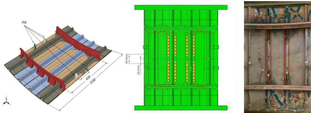
Figure 1: Generic composite A/C fuselage panel: Left – Design; Middle: Schematic with the 4 ribbon tapes, each with 6 FBGs; Right: Complete painted part with the designated locations (4 vertical lines) of the standard polyimide coated single mode fibers used for the distributed sensing.
