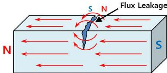
Figure 1: Principle of magnetic flux leakage
