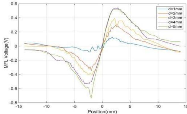
Figure 7: MFL Voltage due to the Defect Depth( $v=3.6\text{km/h}$ )
