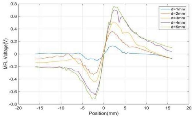
Figure 8: MFL Voltage due to the Defect Depth( $v=7.2\text{km/h}$ )
