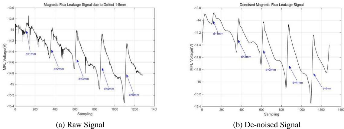
Figure 6: Measured magnetic flux signal from damaged rail specimen
