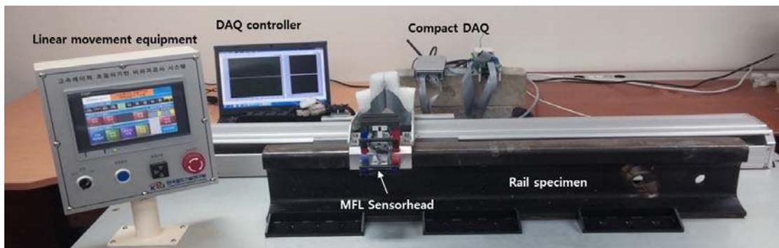
Figure 4: Test setup for railroad track inspection
