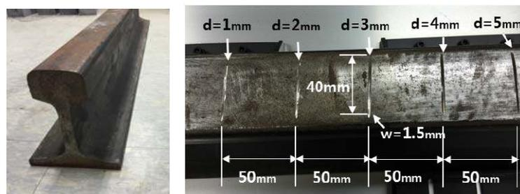
Figure 5: Rail specimen for experiment
