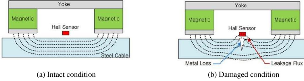
Figure 2: The concept of MFL-based damage detection technique
