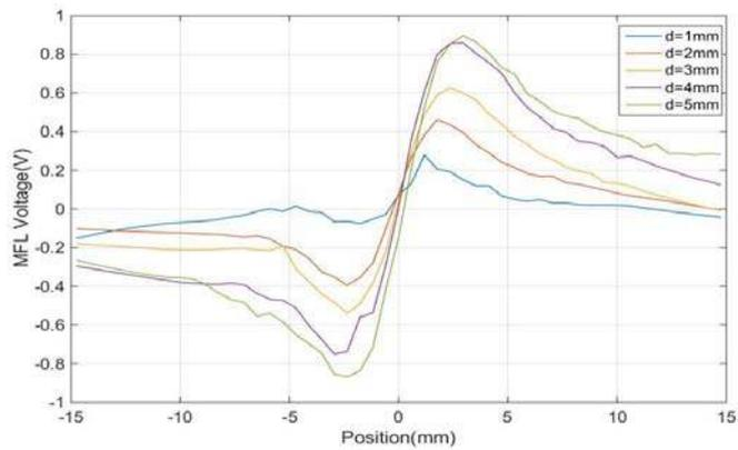
Figure 9: MFL Voltage due to the Defect Depth( $v=10.6\text{km/h}$ )
