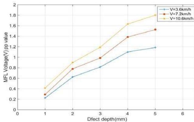
Figure 10:  $MFL_{pp}$  due to the Defect Depth for each Inspection Velocity
