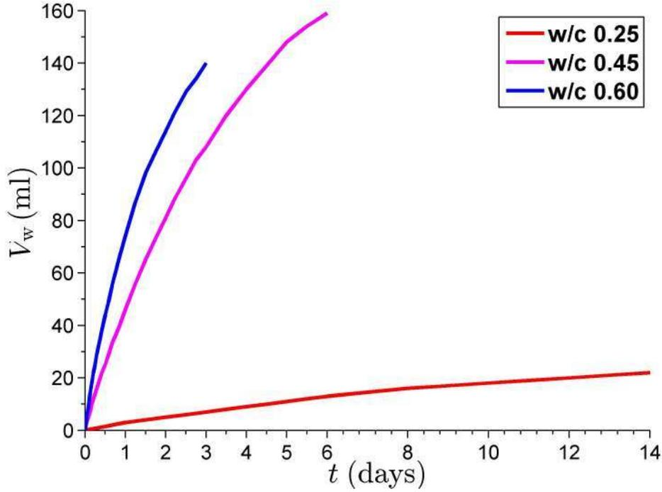
Figure 4 : The absorbed water volume  $V_w$  as functions of time for the mortar specimens with w/c ratios 0.60 (blue), 0.45 (purple) and 0.25 (red).
