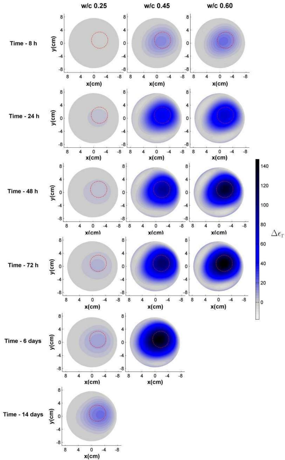
Figure 5 : The evolutions of the relative permittivity change reconstructed based on ECT. The columns from left to right correspond to w/c ratios 0.25, 0.45 and 0.60. The times of the ECT measurements are shown on the left side of each row. The dashed red circle indicates the location of the water reservoir.
