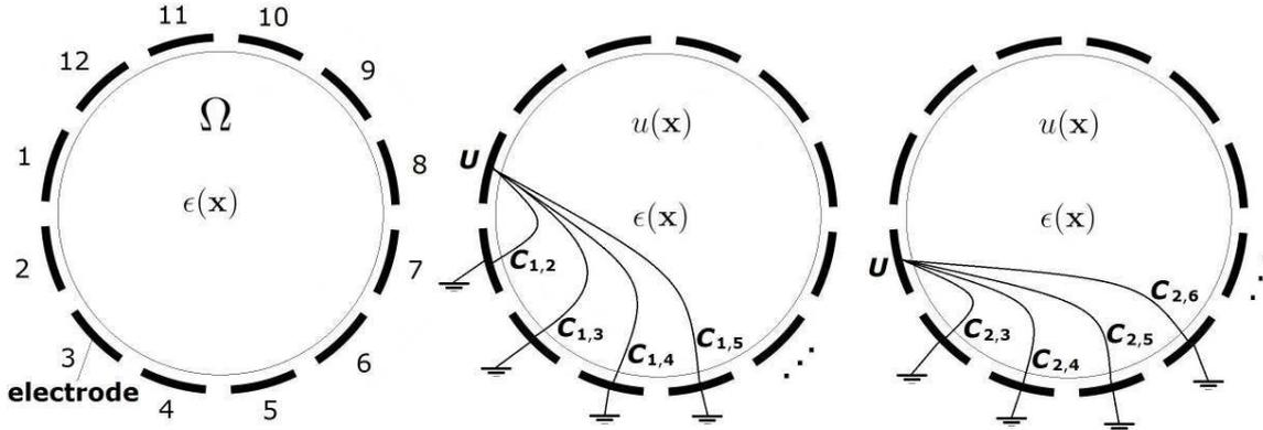
Figure 1 : Left: Illustration of an ECT experiment. Middle and right: Capacitance measurements corresponding to two potential excitations.
