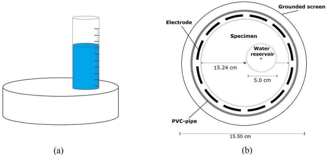
Figure 2 : (a) Schematic illustration of a specimen and a water reservoir. (b) Schematic top-view illustration of the ECT setup and specimen (not to scale).
