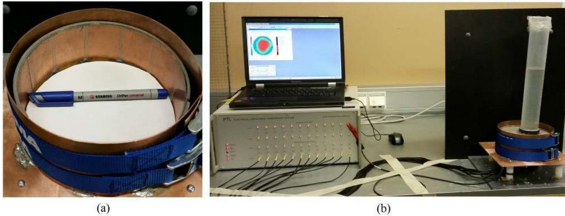
Figure 3 : (a) An empty ECT measurement fixture. (b) PTL300E measurement system, and the experimental setup.
